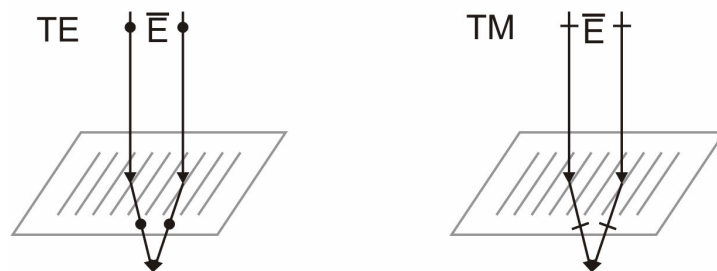
Figure 2.43: Polarisation directions of two interfering beams after passing through a phase mask. In the TE setup the beams are still parallel polarised. In the TM setup the polarisation vectors are no longer parallel but at an angle to each other.
