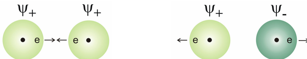
Figure 2.19: Pictorial representation of the formation of orbitals, bonding (left) and antibonding (right).
