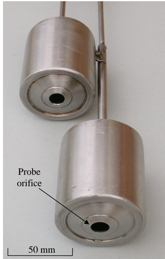
Figure 5.19. Photograph of the large double probes showing the reduced orifice at the base of the probes.
