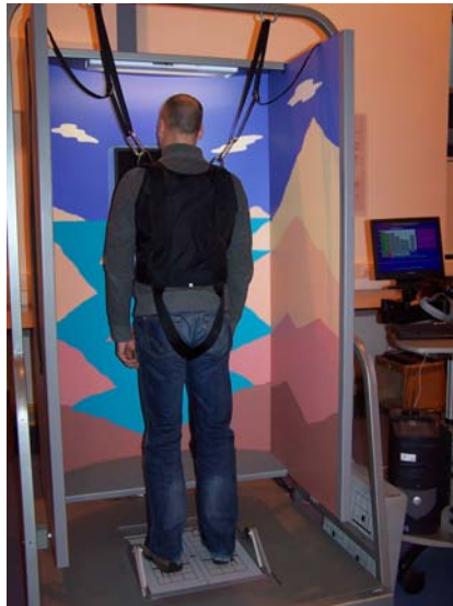
Figure 3.7. NeuroCom Smart Equitest system with sway-referenced moving surround and support surface. The participant is wearing a harness to prevent them from falling during the tests.
