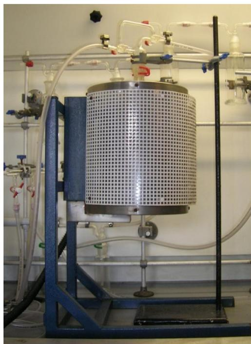
**Figure 2-7.** Representation of the apparatus used in the reactions under  $N_2$  gas.
