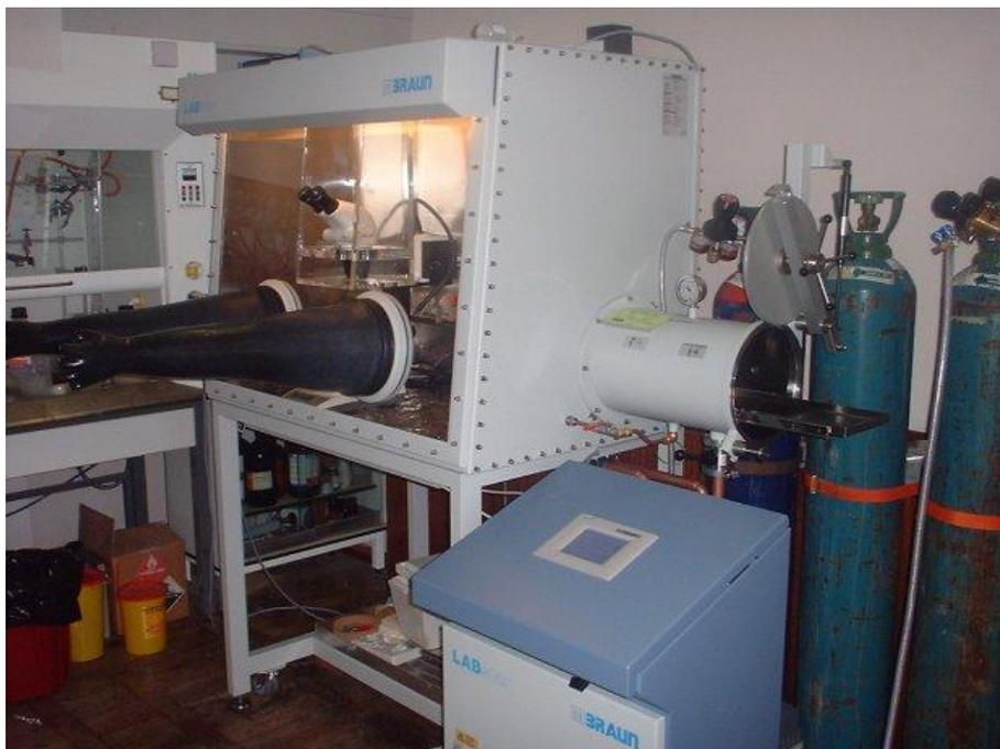
**Figure 2-3.** A M-Braun Lab-Star glove box.
