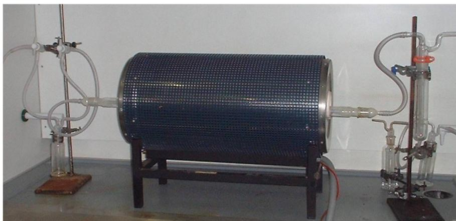
**Figure 2-6.** An example of a tubular furnace.
