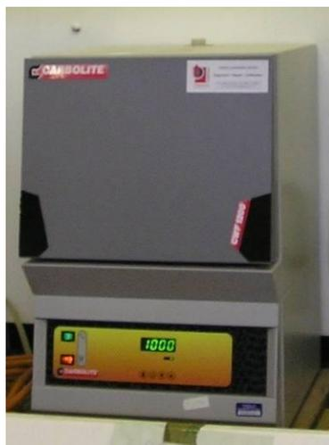
**Figure 2-4.** The Carbolite CWF 1200 box furnace.
