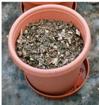
**Figure 2-3: Cylindrical Lysimeter Prototype (C).**
