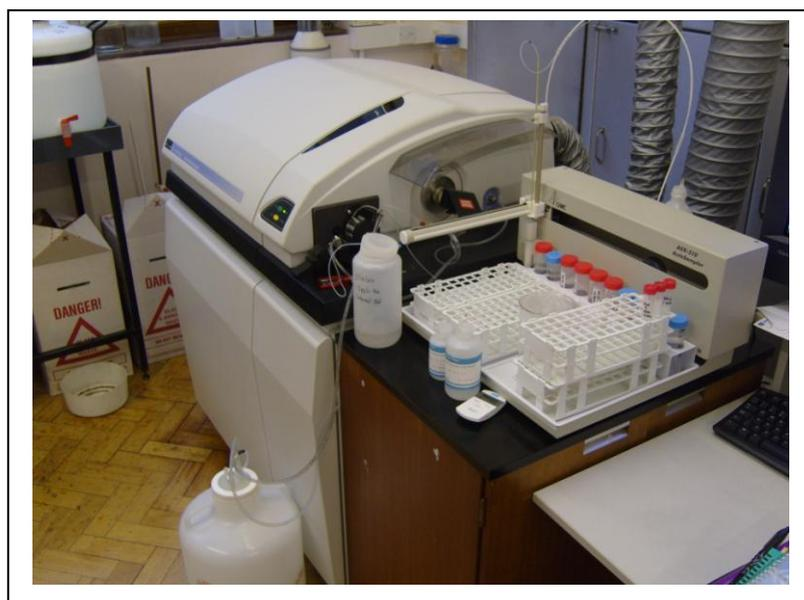
Figure 3-7: ICP-MS Unit
