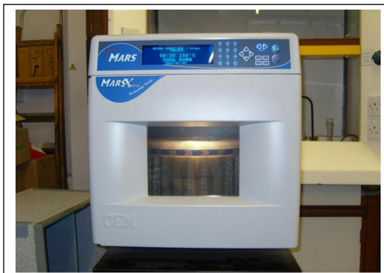
**Figure 3-3: Microwave Digestion**
