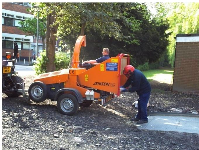
**Figure 2-8: Chipping of Blank Wood and CCATWW**
