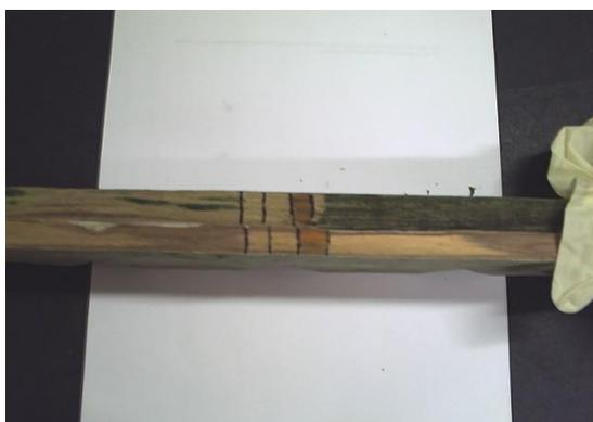
**Figure 2-7: Colour Indicators for CCATWW. PAN stain for Cu is positive (orange) on the right and stannous chloride stain for As is negative on the left**
