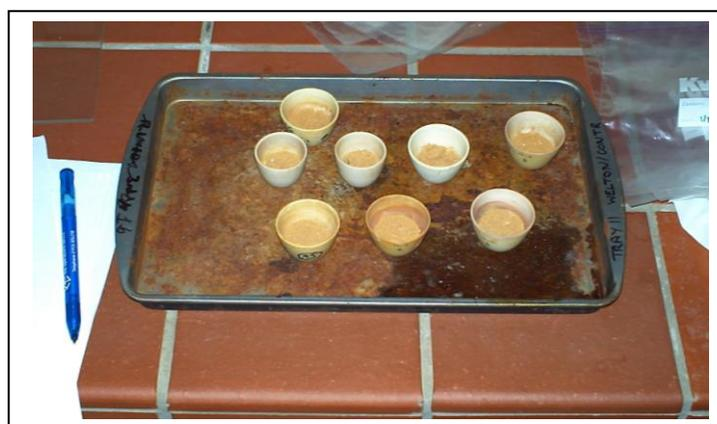
Figure 3-1: Samples Following Loss on Ignition
