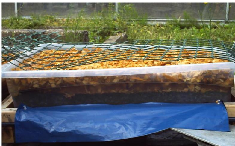
**Figure 2-10: Waterlogging in a Lysimeter**
