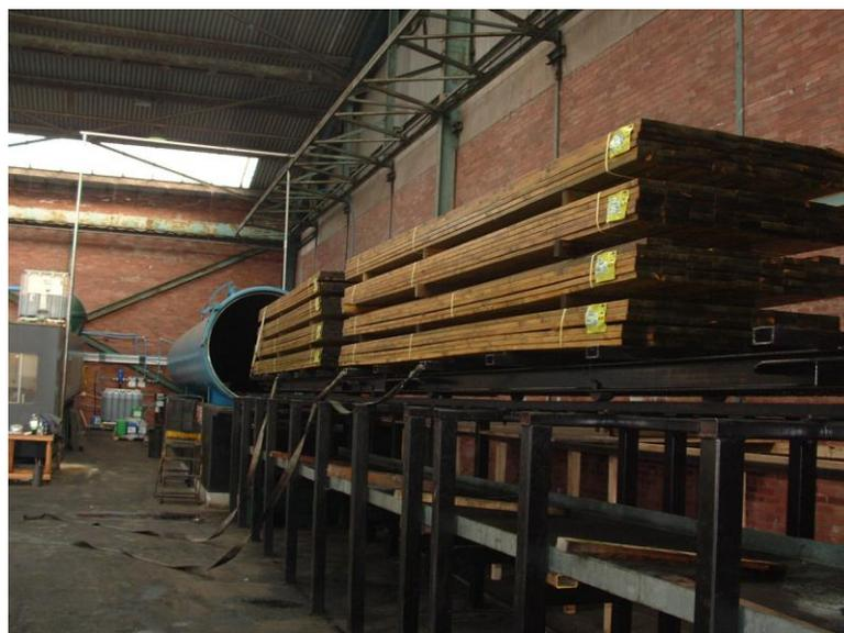
Figure 1-1: Wood Being Removed From a Pressure-treatment Cylinder (courtesy of WJ Components, Hull)
