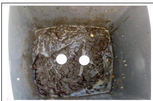
Figure 2-13: Set-up of Soil DGT Mouldings
