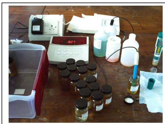
**Figure 3-2: Measurement of pH on Leachate Samples**
