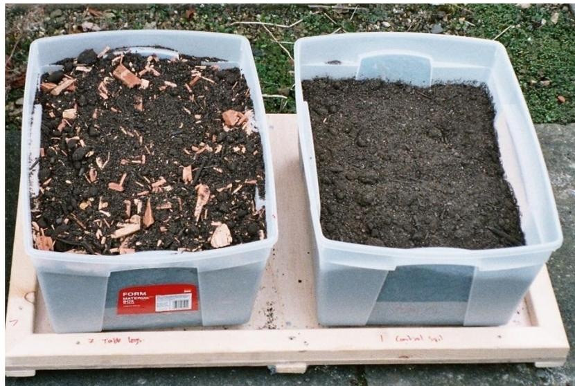
**Figure 2-2: Smaller Lysimeter Prototype (B).**
