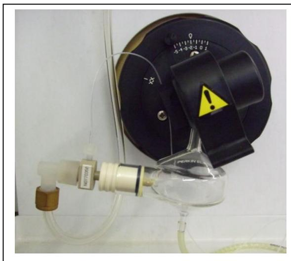
**Figure 3-6: Nebuliser and Vortexing Spray Chamber (courtesy of Bob Knight, 2007)**
