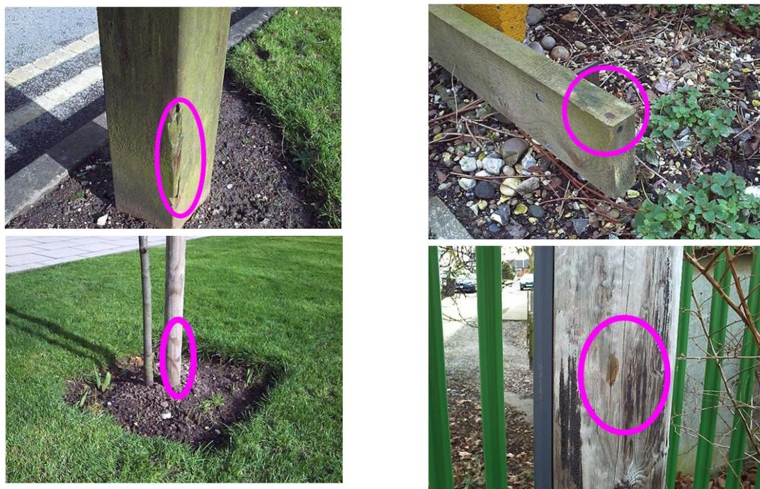
**Figure 2-6: Indicator Techniques for the Presence of Copper in Treated Wood. PAN stains orange and CS stains a deep blue. Results were negative for the stannous chloride test for arsenic**
