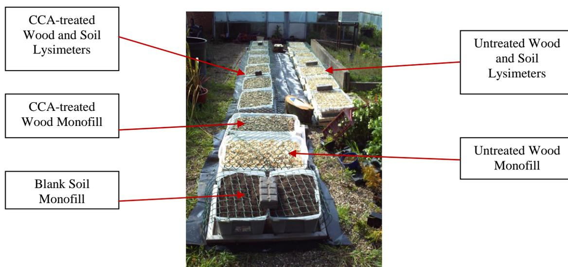
Figure 2-9: Long-Term Leaching Experiment Layout
