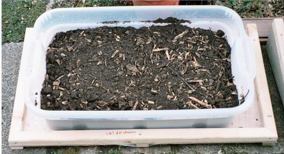
**Figure 2-1: Largest Lysimeter Prototype (A).**
