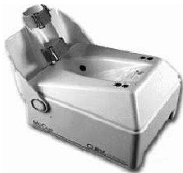
Figure 2.5: The McCue CUBAclinical QUS device for measuring BUA at the human calcaneous (heel)
