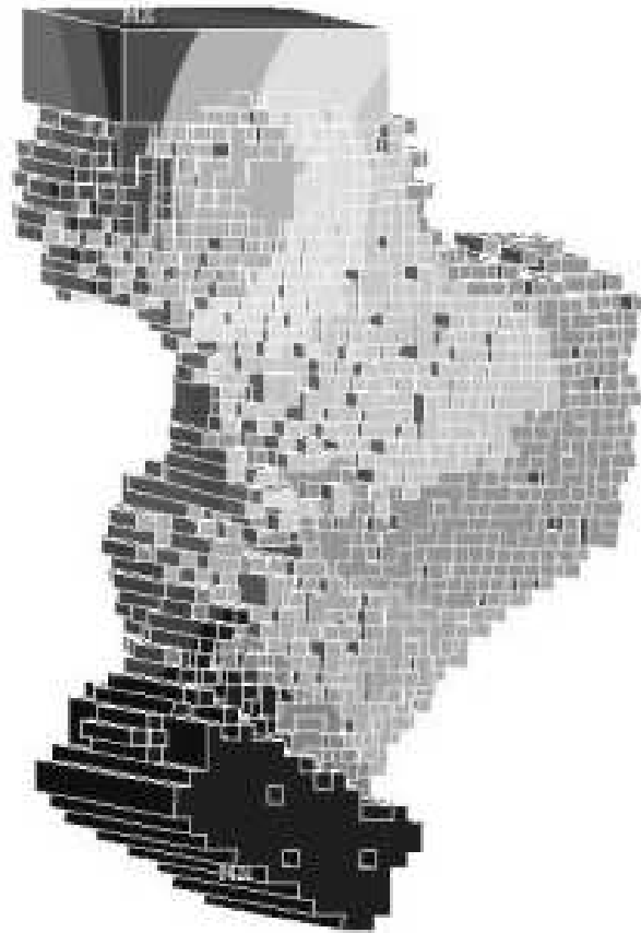
Figure 7.3: Displacement plot for 3D FEXI in stance loading
