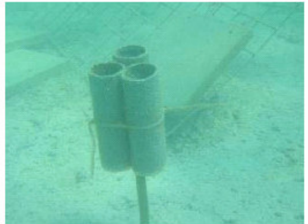
Figure 2.10: Sediment trap design used for sedimentation rate study.
