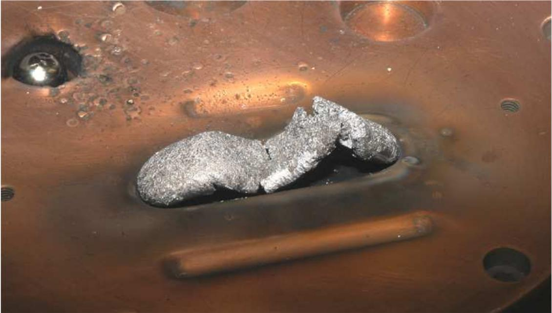
**Figure 4.30** Ingot of  $\text{Fe}_{30}\text{Ga}_{70}$  after arc melting under Argon and cooling
