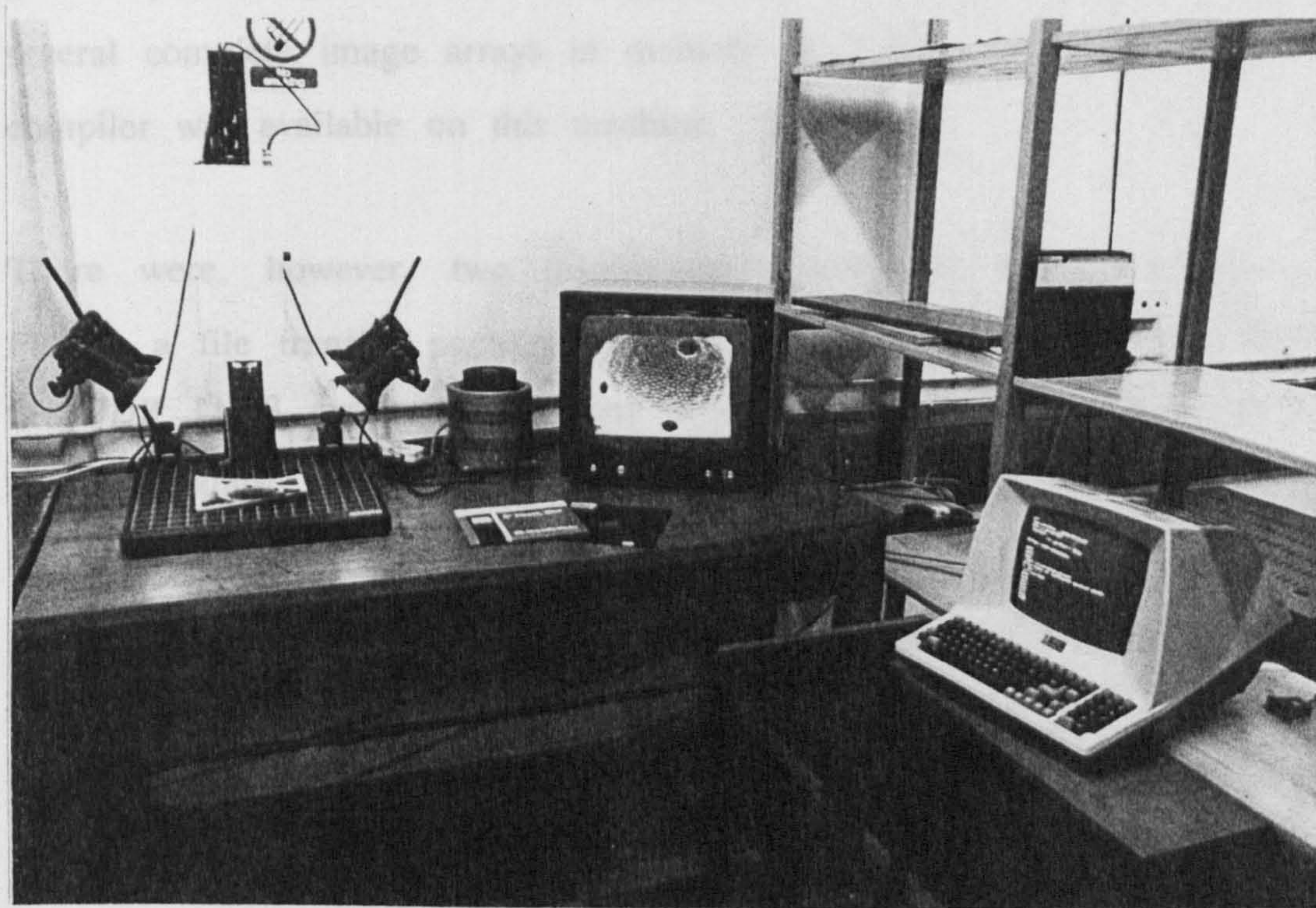
Plate 3-II The equipment used to digitize pollen images. This consisted of a video camera for viewing the photomicrographs, attached to a Matrox frame store and display device. These were all under the control of a DEC PDP 11/23 computer.
