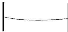
Figure 6.1 Reduction in span after firing.
