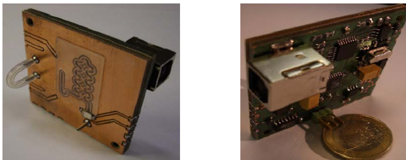
Figure 2 Gaßmann [3] fluidic PCB's
