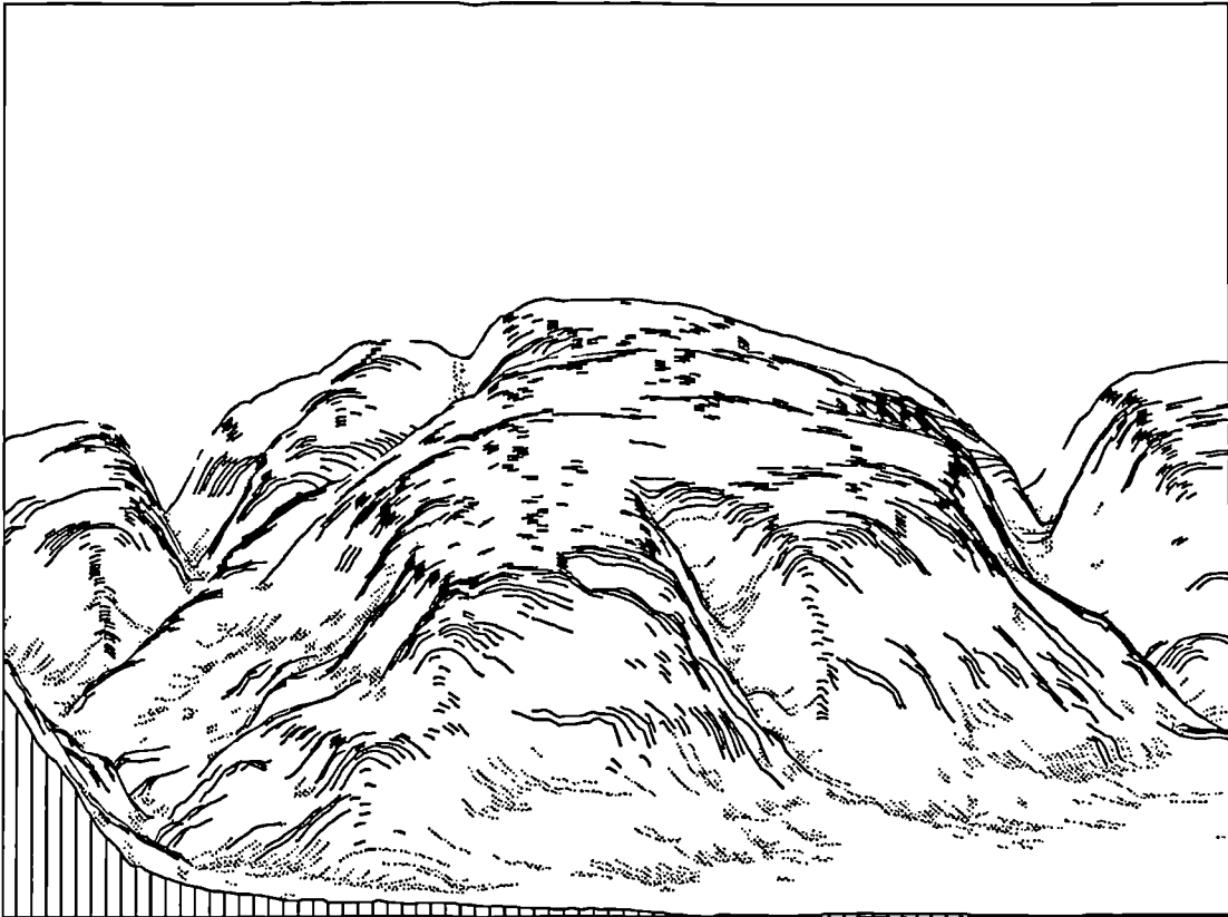
Figure 4.6(b): Sketch of Port Talbot DEM from the west, based on core cells selected by Visvalingam's algorithm using perpendicular distance metric.
