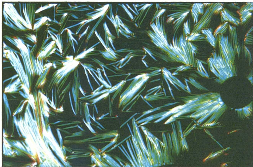
Plate 23. The Filament Texture Exhibited by ( S )-2-Chloro-4-methylpentyl 4'-(4-nonyloxybenzoyloxy)-4-biphenylcarboxylate (158) on Heating from the Smectic A Phase.
