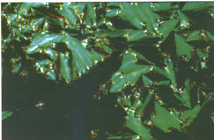
Plate 3. The Broken Focal-Conic Texture of the Smectic C* Phase Displayed by (S)-2-Chloro-4-methylpentyl 4'-(4-nonyloxybenzoyloxy)-4-biphenylcarboxylate.
