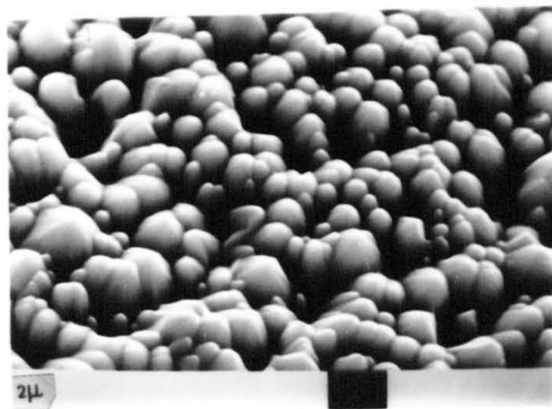
Fig. (5.6): SEM micrograph for a film which had been formed on a smooth substrate of copper, after etching CdS film for 5 seconds. (Viewing angle \sim 30^\circ )
