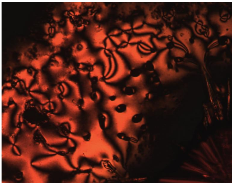
Figure 4. 12: OPM image of 30 in the nematic phase at 164.1°C
