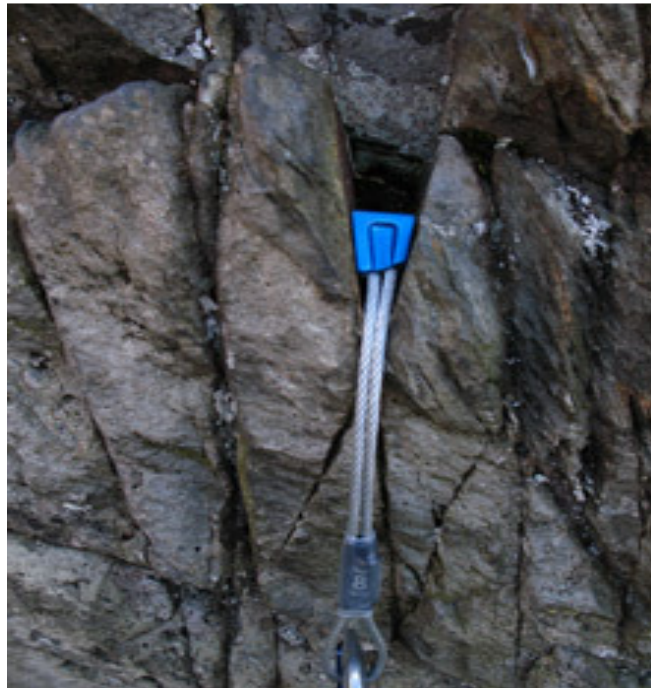
Figure 6.24 A number 8 nut placed in an inverted crack
