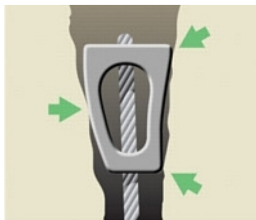
Figure 6.22 Diagram showing the forces placed on a nut (source www.wildcountry.co.uk )
