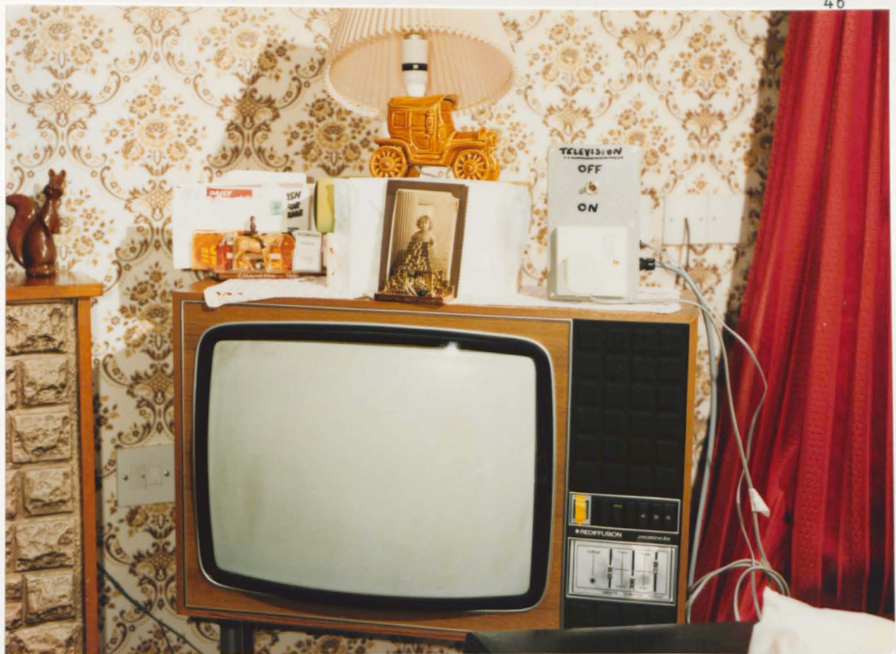
2:10 Switch for TV to enable recording of on-time
