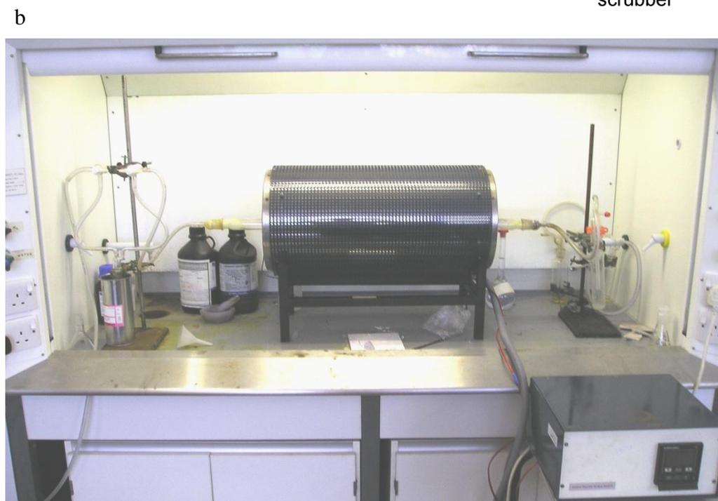
**Figure 2.1** a) Diagram of the apparatus used for reactions of solids with  $\text{CS}_2$  vapour. b) Tubular furnace used in sulphuration reactions
