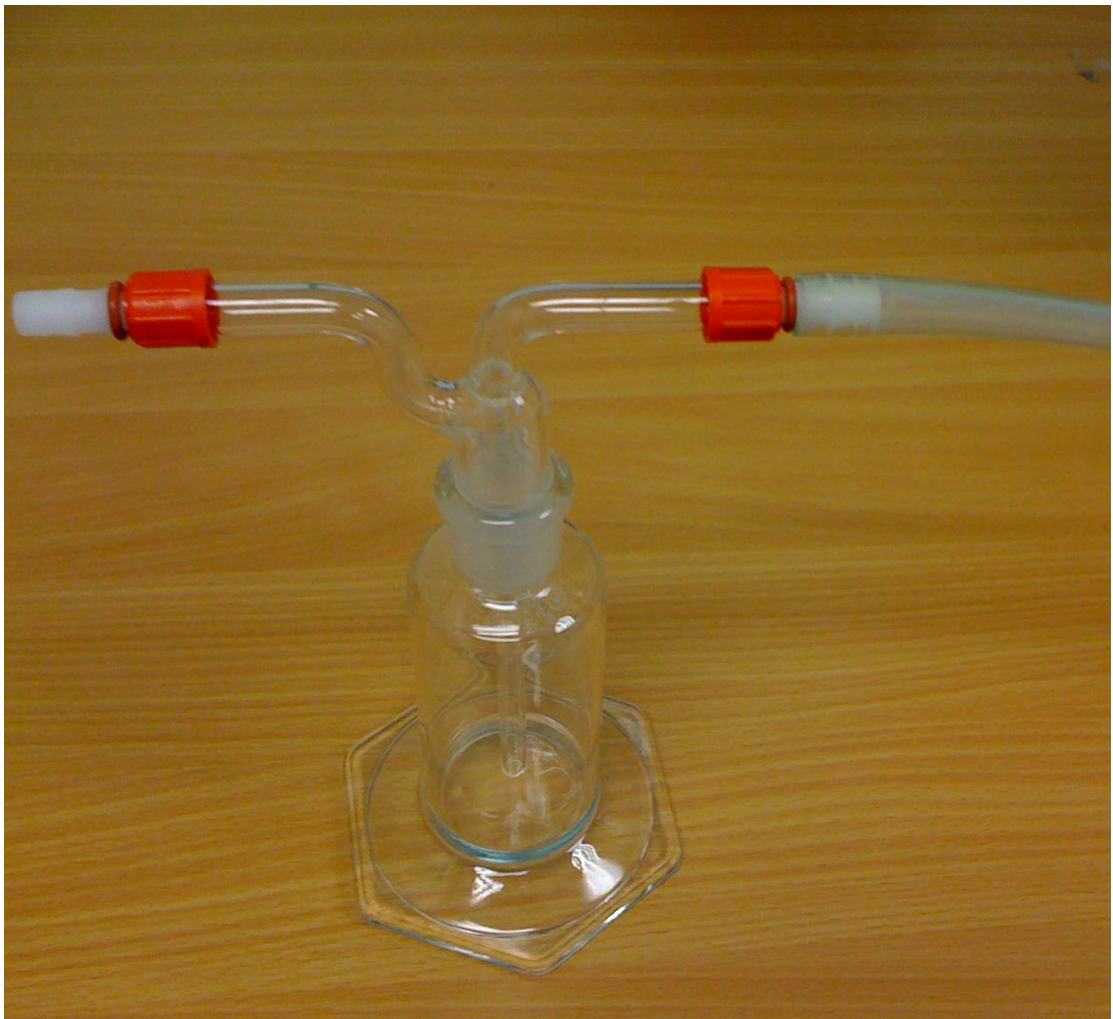
Figure 2.6 Exhaled breath condensate device used for the collection of sample. A nose clip was used and 1-2 ml of sample was obtained after 10 minutes of normal tidal breathing. The device was kept in an ice box during the collection.
