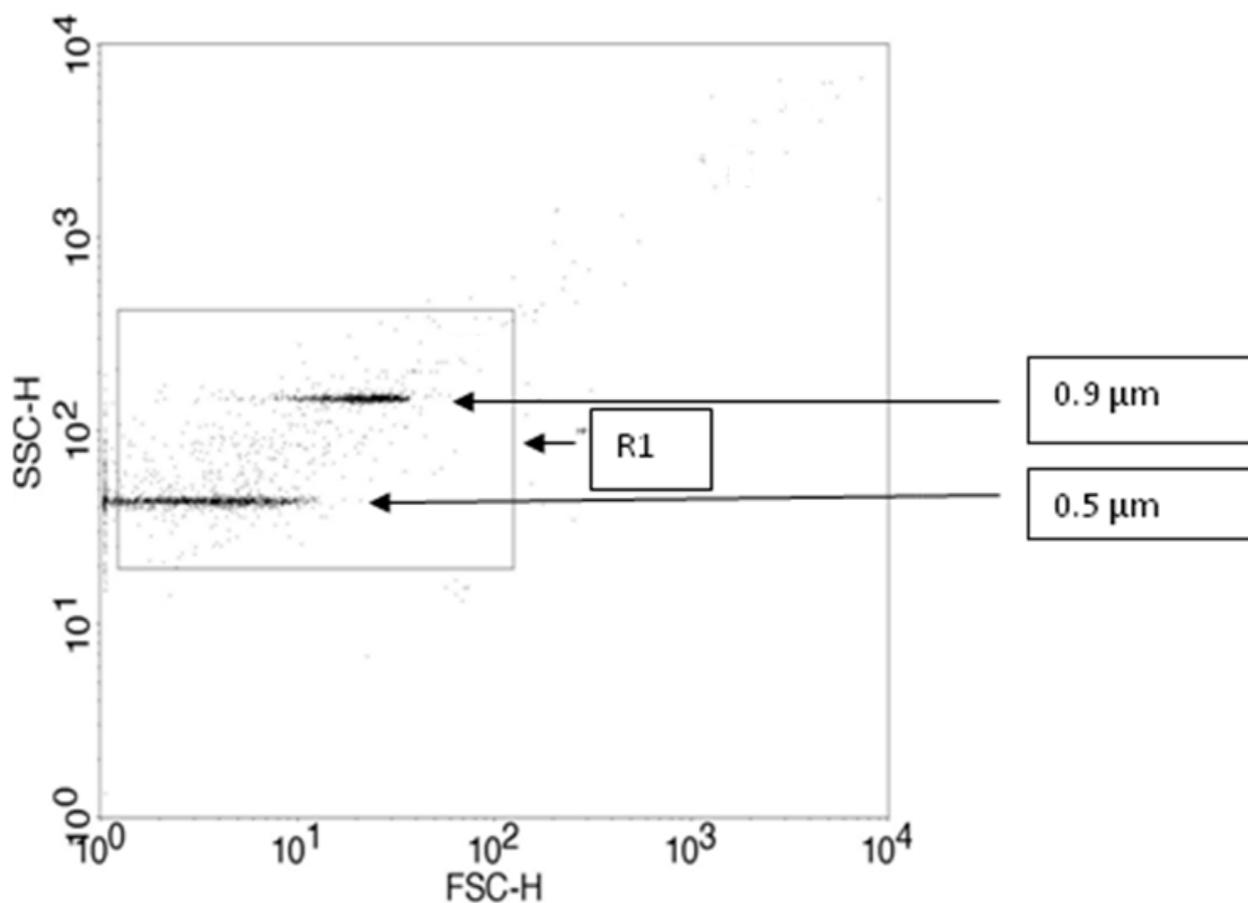
**Figure 8.1:** A dot plot of Forward scatter (X axis) and Side scatter (Y axis) for a megamix beads sample 0.5  $\mu\text{m}$  and 0.9  $\mu\text{m}$  diameters. MP will be expected within the quadrant box defined as R1.
