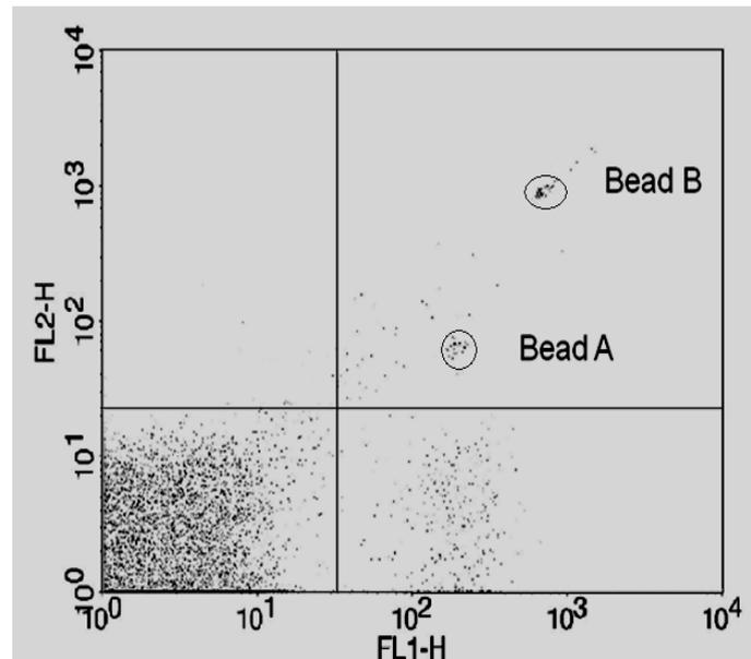
**Figure 8.2:** A dot plot with CALTAG counting beads was determined. There are two beads in the right upper quadrant, bead A (685) and bead B (667). The negative control is in the lower left quadrant. The expression of FITC marker is in the right lower quadrant. The PE expression is in the upper left quadrant. Dual FITC/PE stained MP will be in the upper right quadrant.
