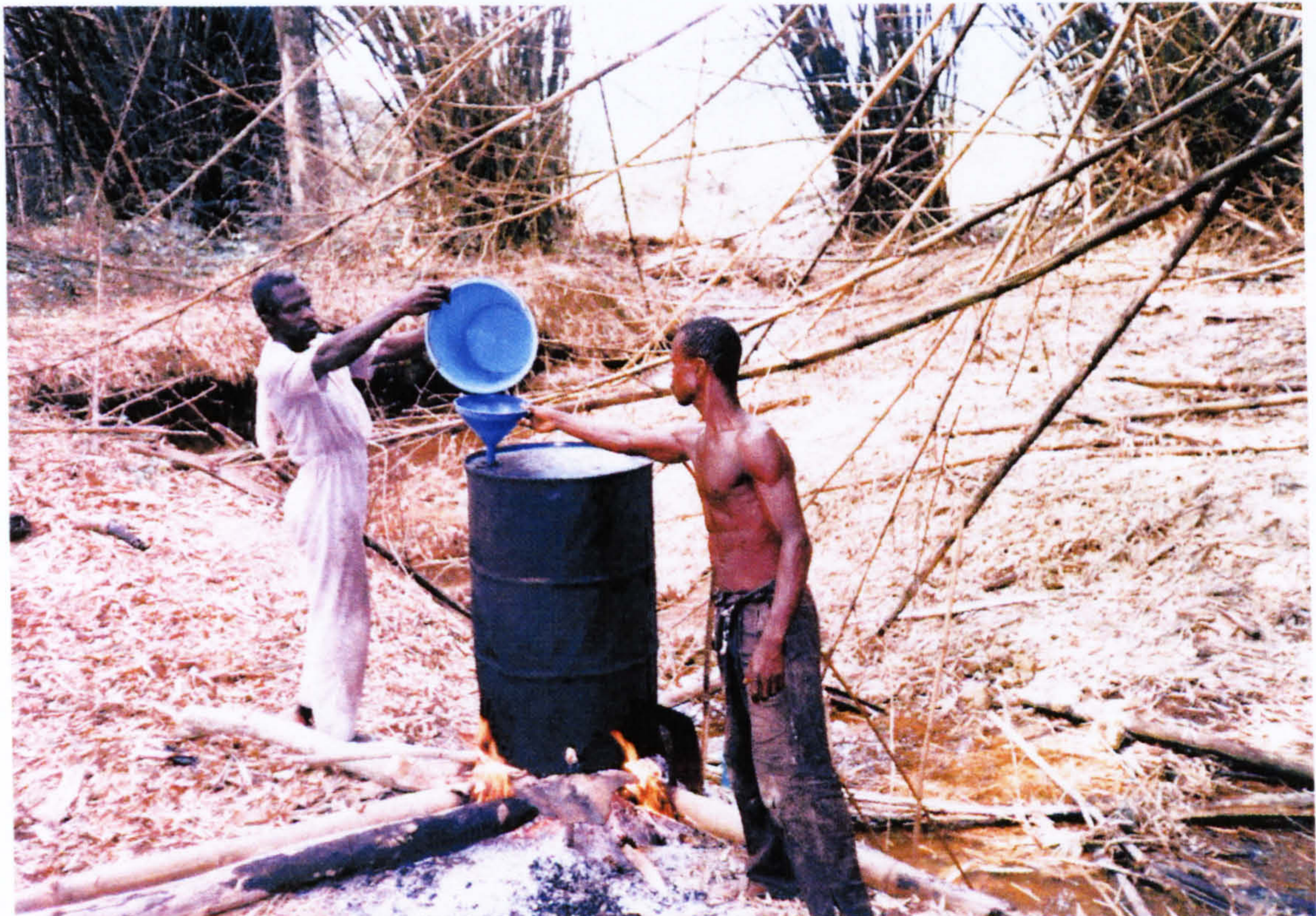
Plate 6.2: 'Akpeteshie' distilling camp. Palm wine tapped from raphia and oil palm is distilled to produce a local gin called 'akpeteshie'.
