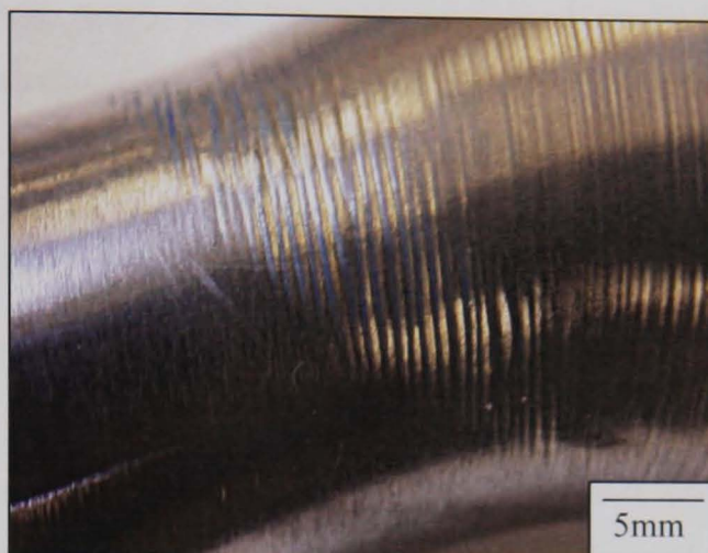
Figure 6.17 : Optical images of the ‘eye’ shaped area of flow-like grooves, generated under standard wear conditions, against a discharge pressure of 6 bar, on the rotor
