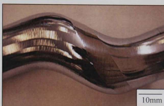
Figure 6.21 : Exposed substrate on the leading edge of a hard chromium plated rotor tested under standard test conditions with a 45 micron silicon carbide slurry
