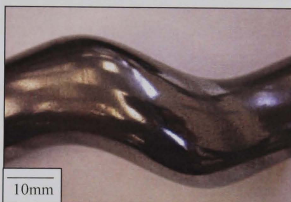
Figure 6.20: Tungsten carbide rotor tested under standard test conditions with a 45 micron silicon carbide slurry
