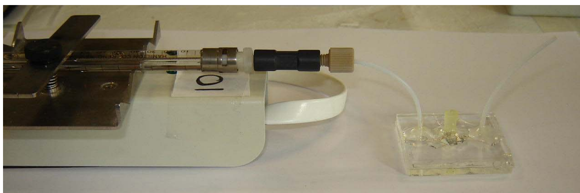
Figure 99. Experimental setup for the microreactor synthesis of theaflavin
