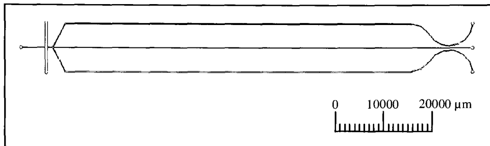
Figure 2-17 Micro-fluidic device design 8: Channels are etched to a depth of 50 μm, vertical channel widths of 600 μm and the separation channel has a width of 200 μm.
