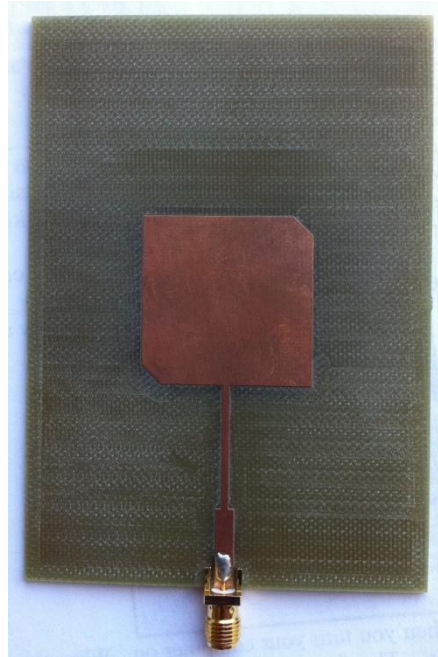
Figure 3.15. The fabricated conventional corner truncated CP SP antenna
