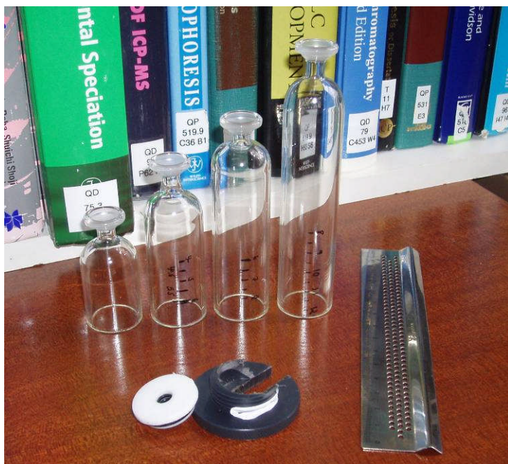
Figure 4.14 Image of 4 chambers used in evaporation chamber length optimisation. No drain provided in chamber. Also showing PTFE adapter to hold MicroMist nebuliser (white) and adapter to secure chamber to Elan DRC II torch (grey), both fabricated by departmental workshop.
