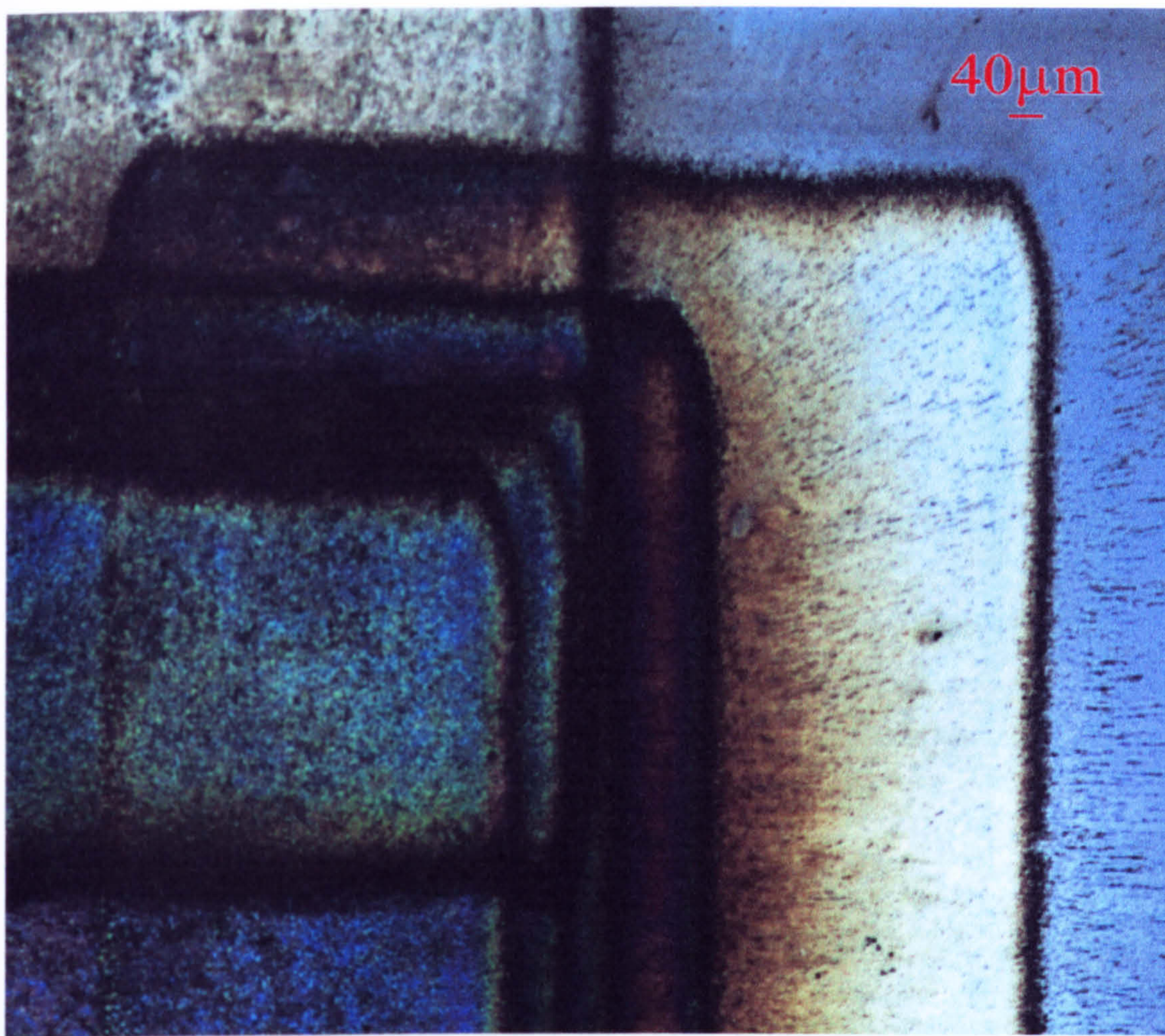
Figure 6.21 Six overlapping transferred layers of ZnS film. The lowest one extends more to the right, two more are over its left part, then one transversed upwards and two more again being displaced left. The transfers were made with a fluence of 0.63 \text{ Jcm}^{-2} in an argon atmosphere at a pressure of 4.2 \times 10^{-2} \text{ mbar} .
