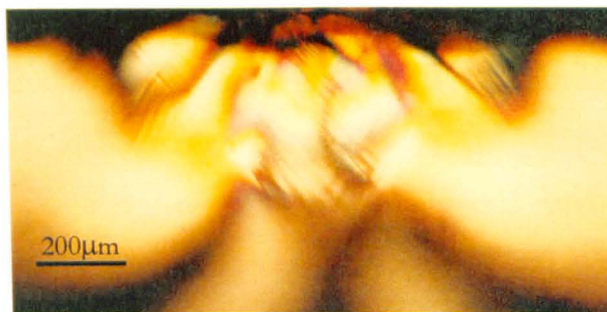
Figure 4.9. Micrograph of the deformed volume of an impression with a rosette formation, taken through a window polished on a (110) perpendicular to the impressed surface.
