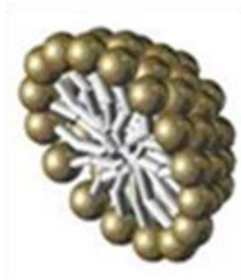
Figure 1.3. Cross-sectional view of a micelle with the hydrophilic head groups on the outside and the “liquid like” hydrophobic core made up of the tail groups.[3]
