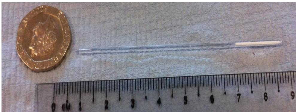
**Figure 2.1** The potassium silicate frit made in the capillary.
