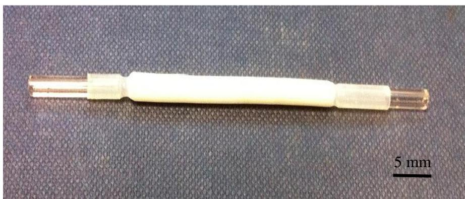
**Figure 4.1** In-house fabricated silica monolithic column sealed within Teflon tubing.
