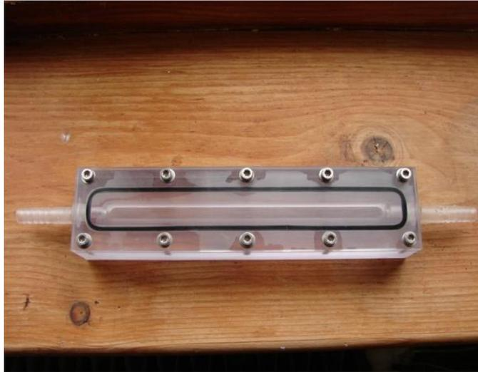
**Figure 4.3 Redesigned microcosm with built in flow channel**
