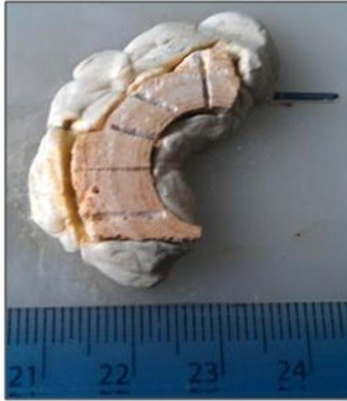
**Figure 3.2** Drilling lines across tufa sample
