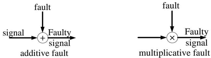
Figure 1-5: Additive fault and Multiplicative fault
