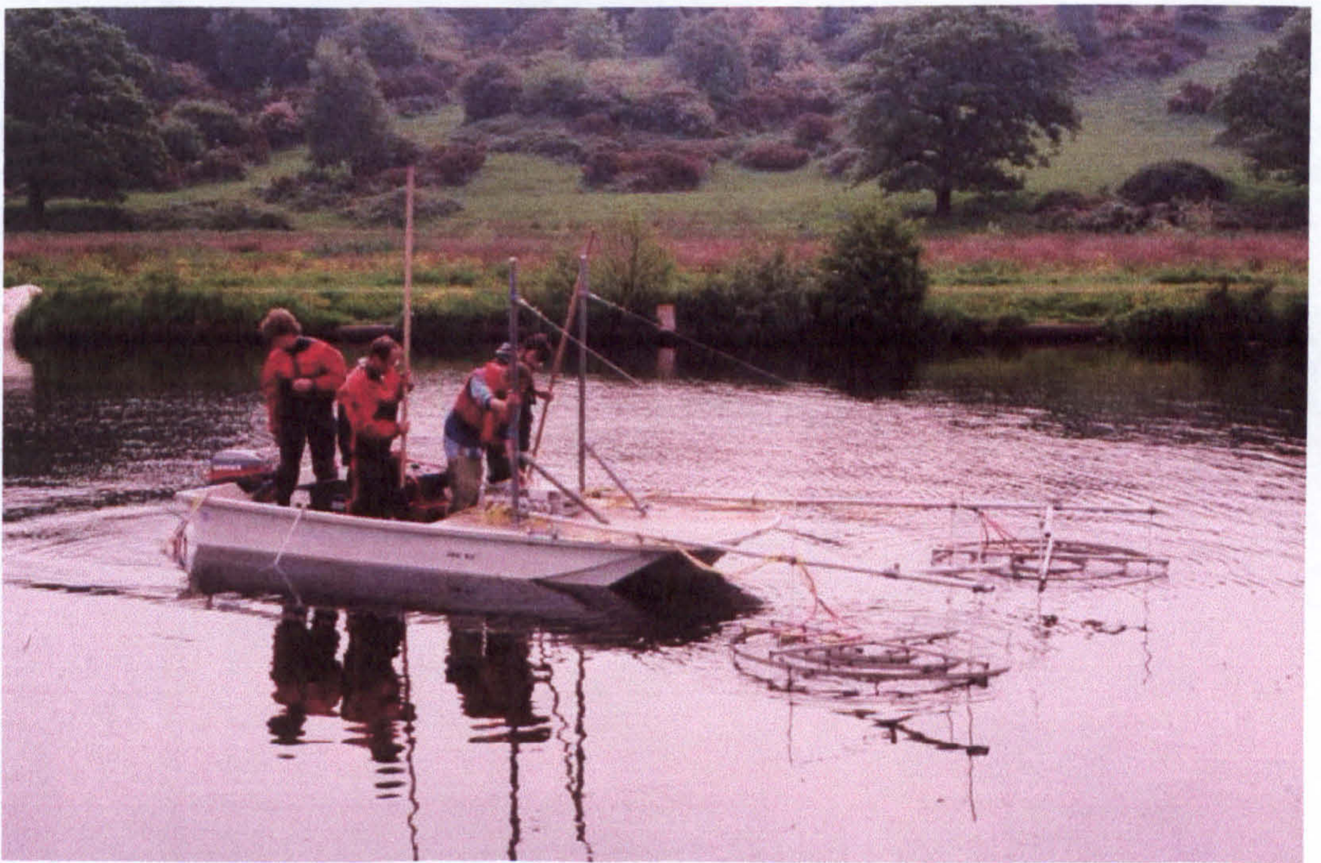
Plate 3.2 Boat mounted electric fishing equipment, displaying the two electrode arrays, each consisting of three concentric metal rings.
