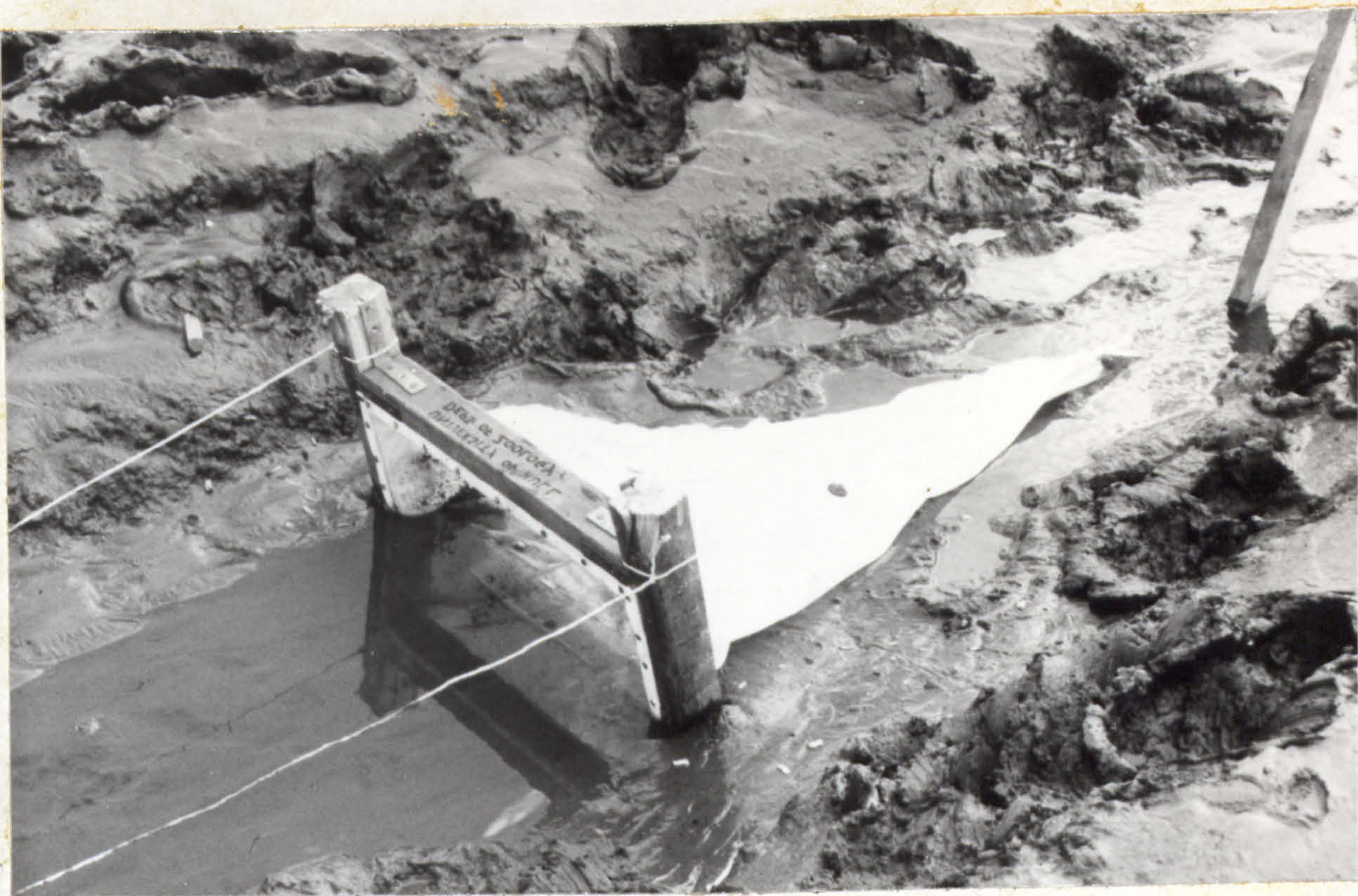
Plate 13 Nekton sampler trap in drainage gully.
