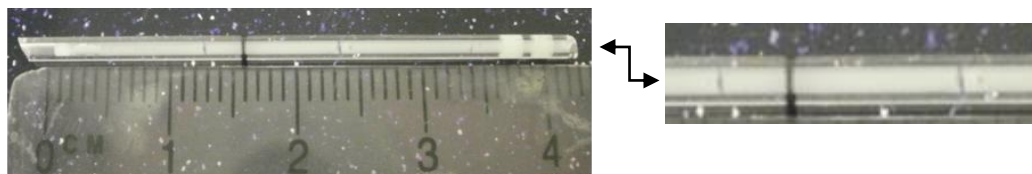
Figure 3.32 The shrinkage phenomena in the silica-based monolith prepared inside the micropipette. The sol-gel precursor was 2.256 mL TMOS, 0.282 g PEO, 2.537 mL 1M \text{HNO}_3 solution, and 0.291 mL distilled \text{H}_2\text{O} .
