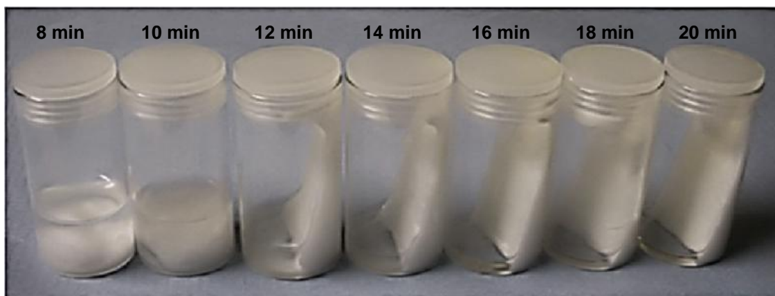
Figure 3.6 Effect of the duration of exposure to the UV lamp on the formation of the poly (BuMA- co -EDMA) monolith.
