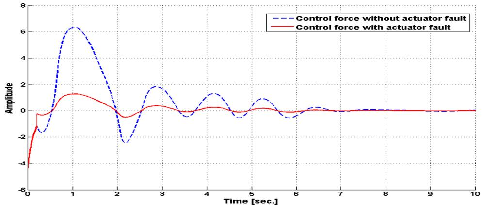
Figure 7-8: Control signal for 80% of 1<sup>st</sup> subsystem actuator fault ( $\eta_1=10$ )
