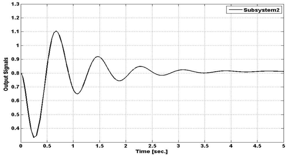
Figure 5-4: Response of 2<sup>nd</sup> subsystem without control
