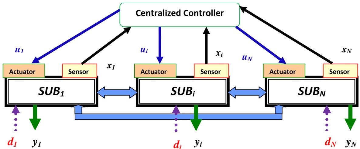
Figure 1-2: Centralized control of inter-connected systems
