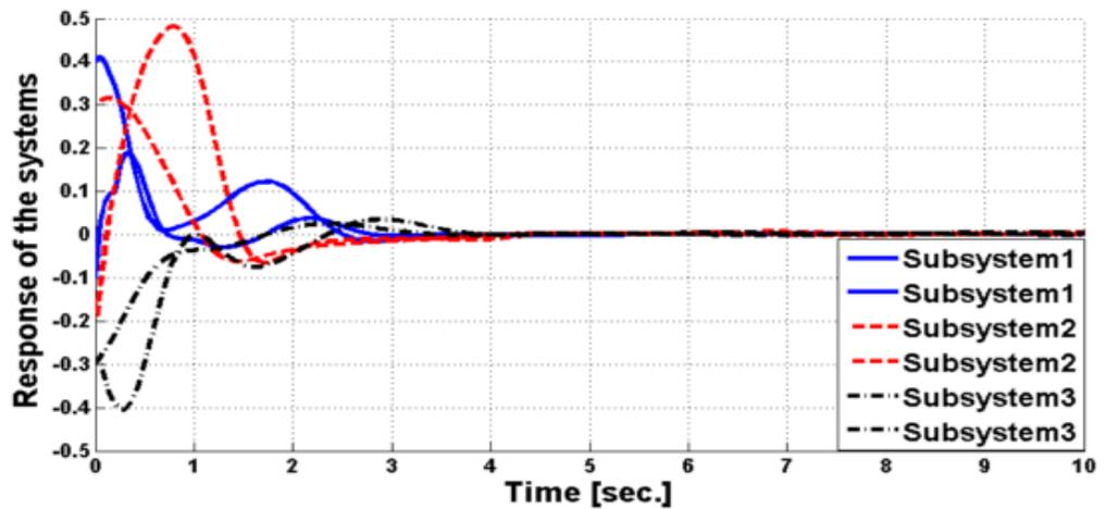
Figure 4-16 : Three subsystems with controls and with 50% actuator fault in 1<sup>st</sup> subsystem
