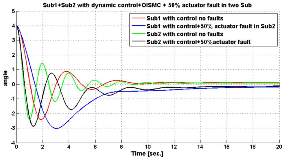
Figure 6-7: Two subsystems with controller and 50% actuator faults in each subsystem
