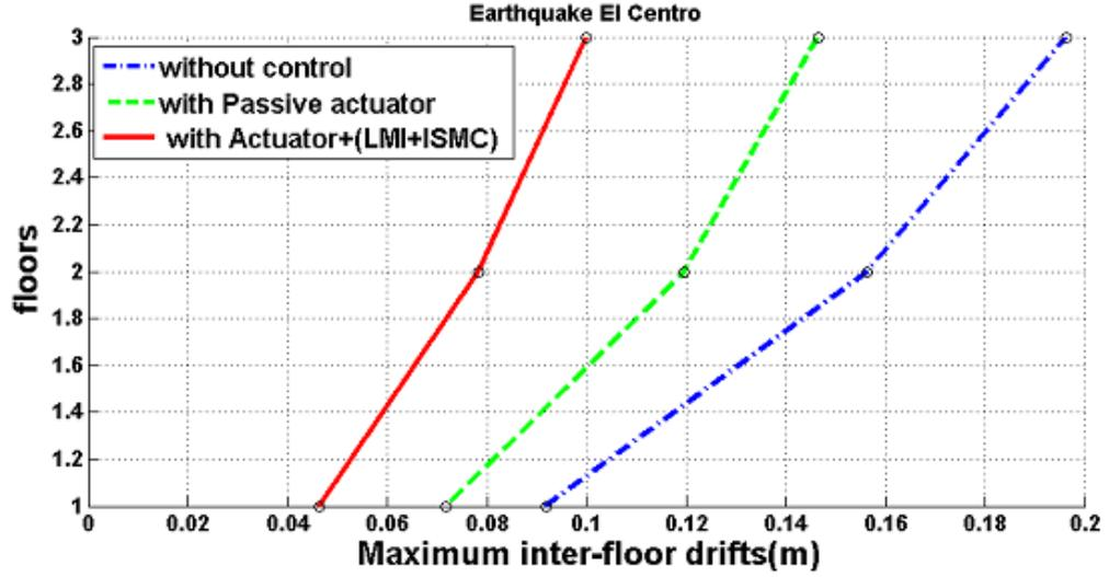
Figure 3-23 : Maximum inter-floor displacement: 1<sup>st</sup>, 2<sup>nd</sup> and 3<sup>rd</sup> floor 70% actuator fault
