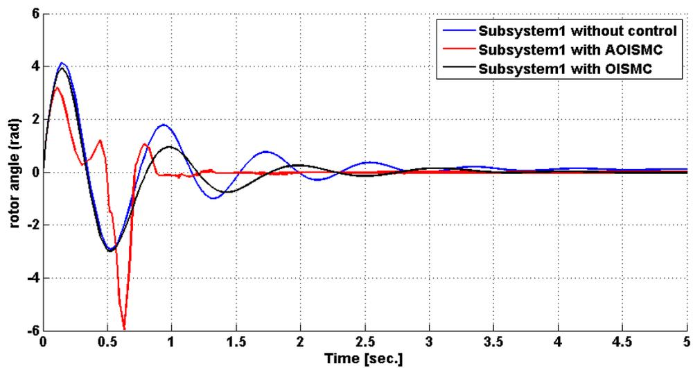
Figure 5-5 : The rotor angle with OISM and AOISM with no fault
