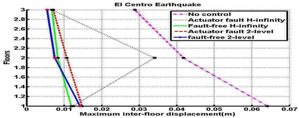
Figure 2-22: Maximum inter-floor displacement: 2<sup>nd</sup> floor actuator fault
