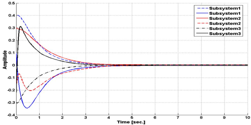
Figure 7-2: Control of inter-connected systems via LMI + ISMC each subsystem individually without any actuator faults
