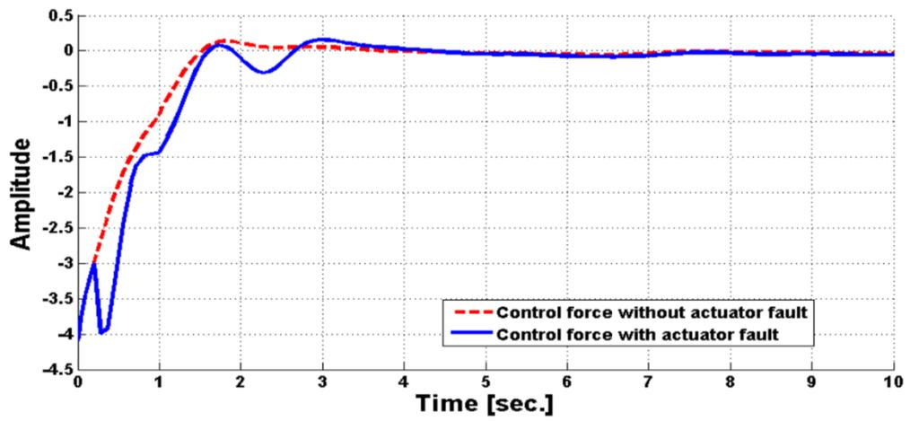
Figure 4-8: Control signal of the 1<sup>st</sup> subsystem with 50% actuator fault
