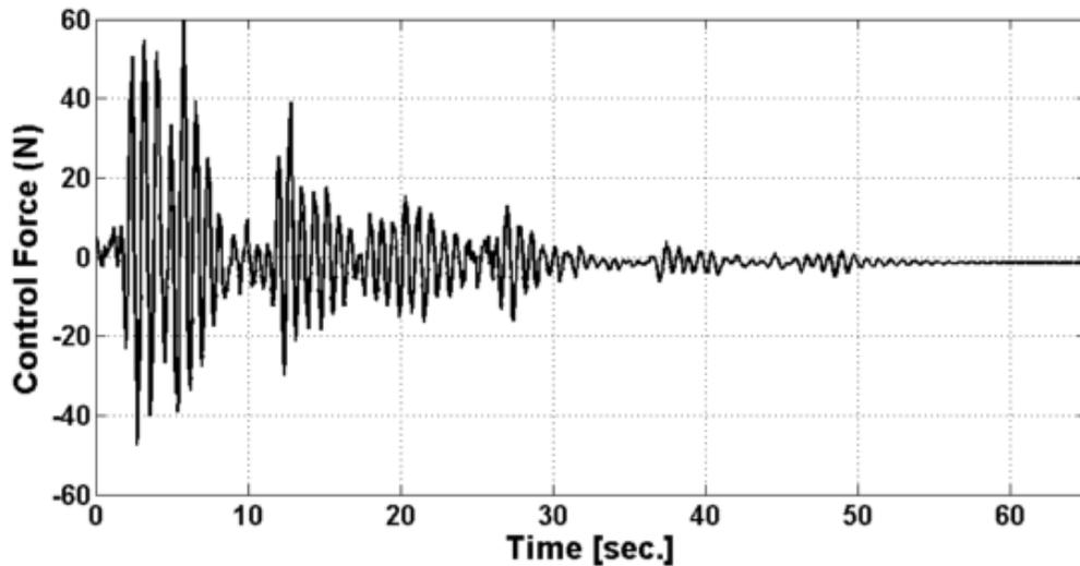
Figure 3-26 : 1<sup>st</sup> floor actuator force with 70% actuator fault
