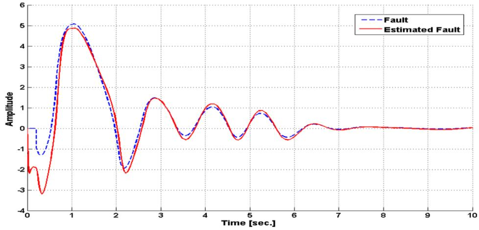
Figure 7-7: Estimated fault for 80% of 1<sup>st</sup> subsystem actuator fault ( $\eta_1=10$ )
