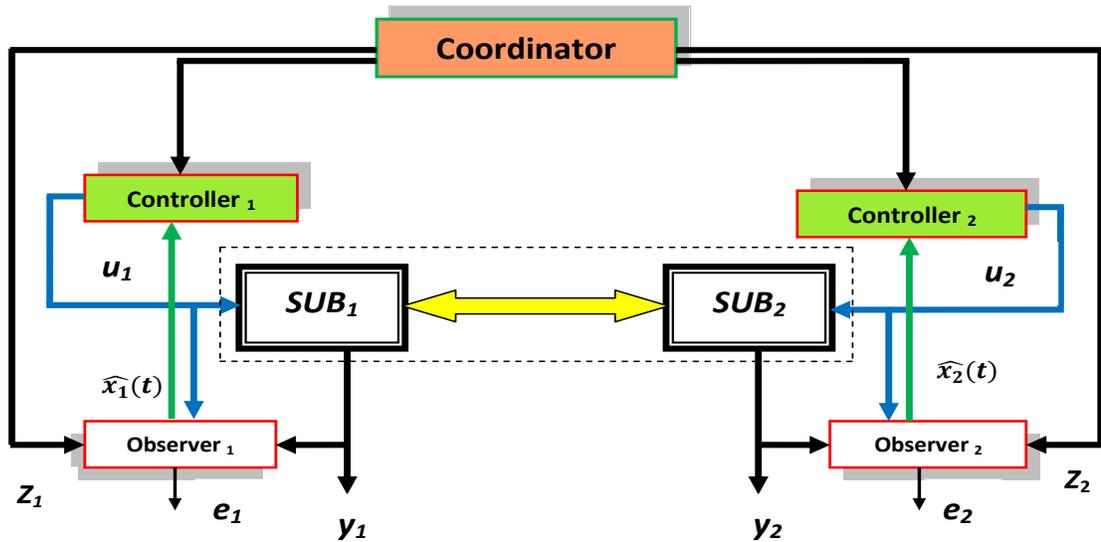
Figure 2-9: Coordinate all the subsystems with its controller and observer
