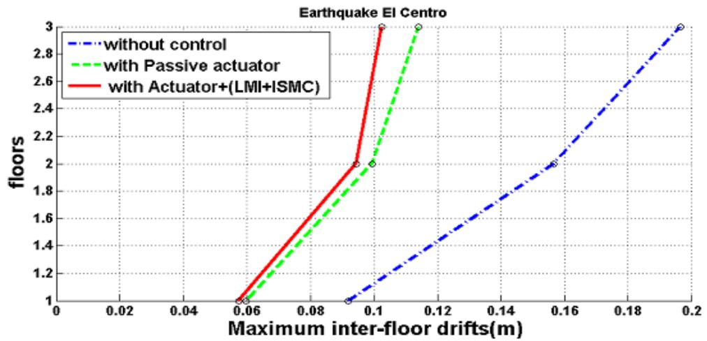
Figure 3-15: Maximum inter-floor displacement: 1<sup>st</sup> and 2<sup>nd</sup> floor 70% actuator fault
