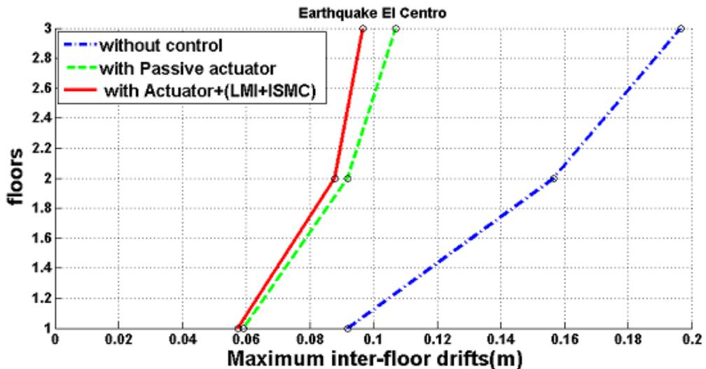
Figure 3-13: Maximum inter-floor displacement: 1<sup>st</sup> floor 70% actuator fault
