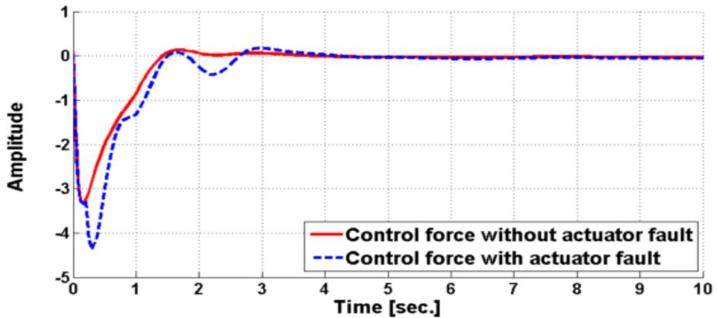
Figure 4-17 : The control signal of the 1<sup>st</sup> subsystem with a 50% actuator fault
