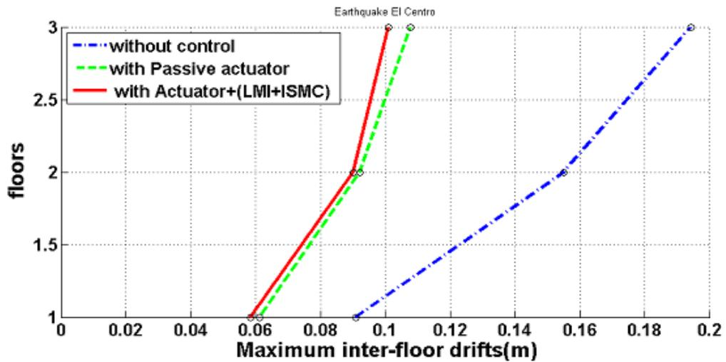
Figure 3-28 : Maximum inter-floor displacement: 1<sup>st</sup> floor 100% actuator failure
