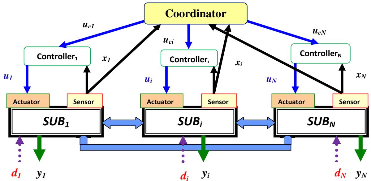
Figure 1-5: Multi-level control of inter-connected systems
