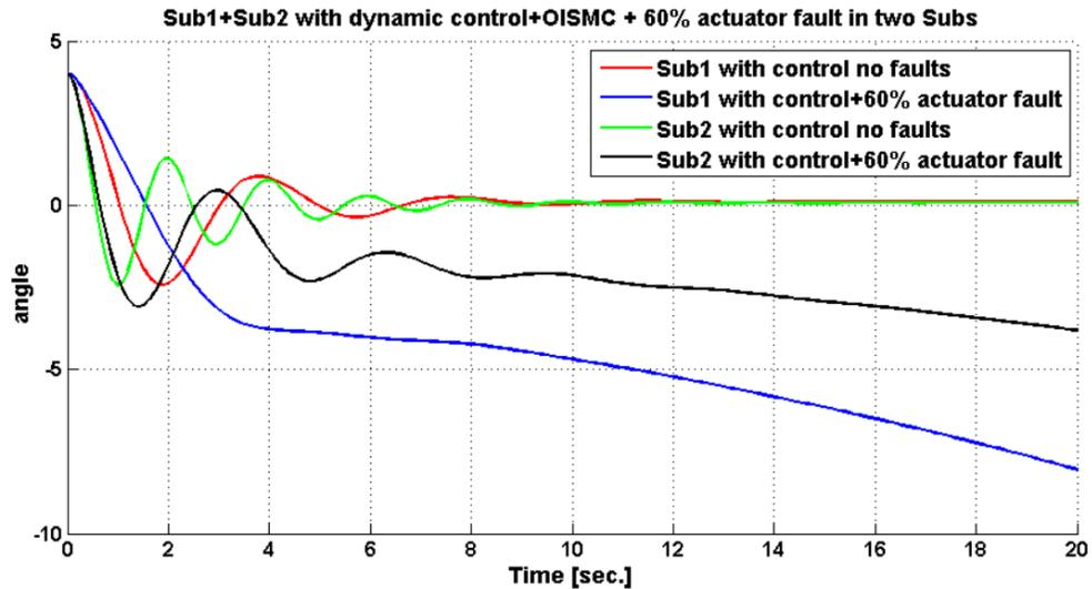
Figure 6-8 : Two subsystems with controller and 60% actuator faults in each subsystem
