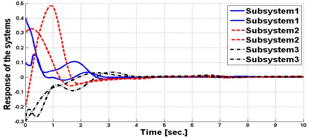
Figure 4-7: Three subsystems with controls and with a 50% actuator fault in 1<sup>st</sup> subsystem
