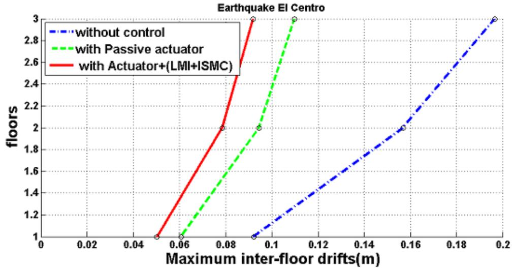
Figure 3-21 : Maximum inter-floor displacement: 1<sup>st</sup> floor 100% actuator failure
