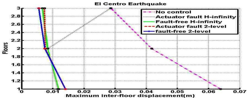
Figure 2-23: Maximum inter-floor displacement: 3<sup>rd</sup> floor actuator fault
