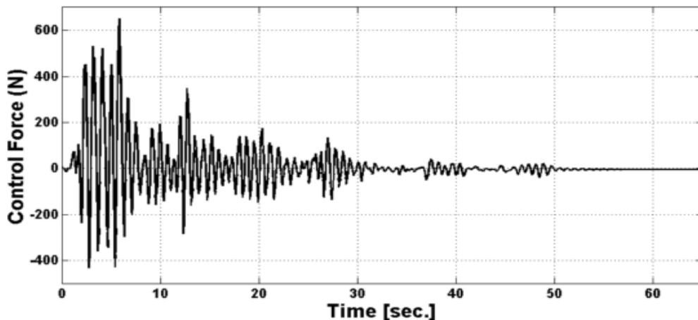
Figure 3-18: 1<sup>st</sup> floor control force with no faults
