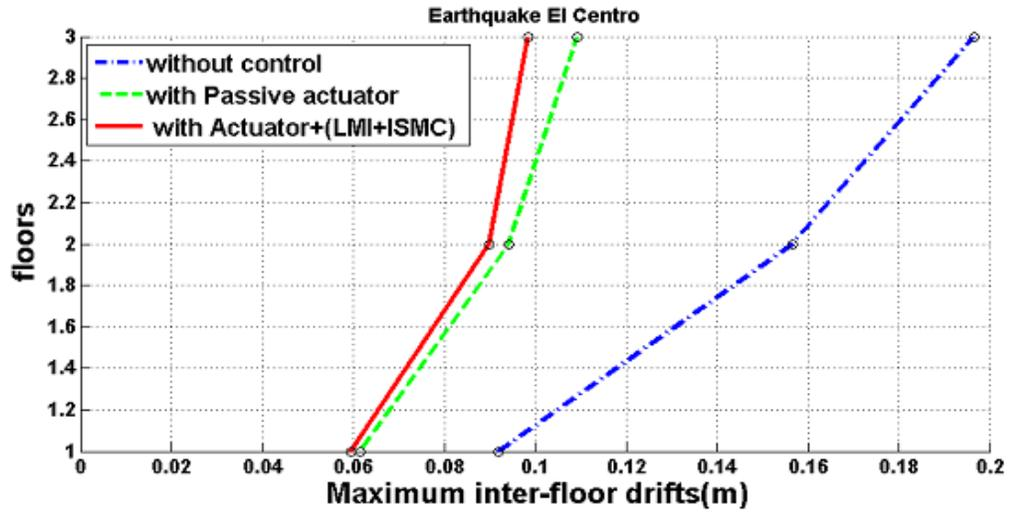
Figure 3-14: Maximum inter-floor displacement: 1<sup>st</sup> floor 100% actuator failure
