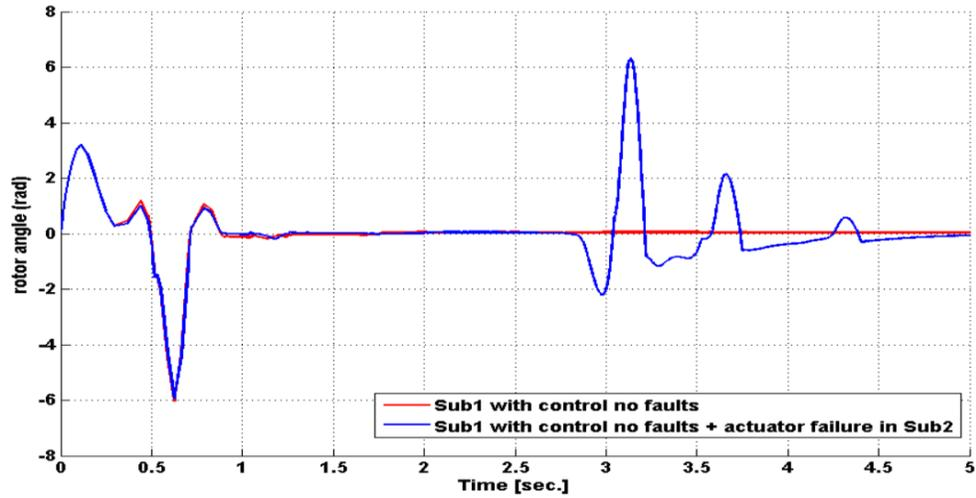
Figure 5-10 : AOISM with 1<sup>st</sup> subsystem fault-free and 2<sup>nd</sup> subsystem with actuator failure
