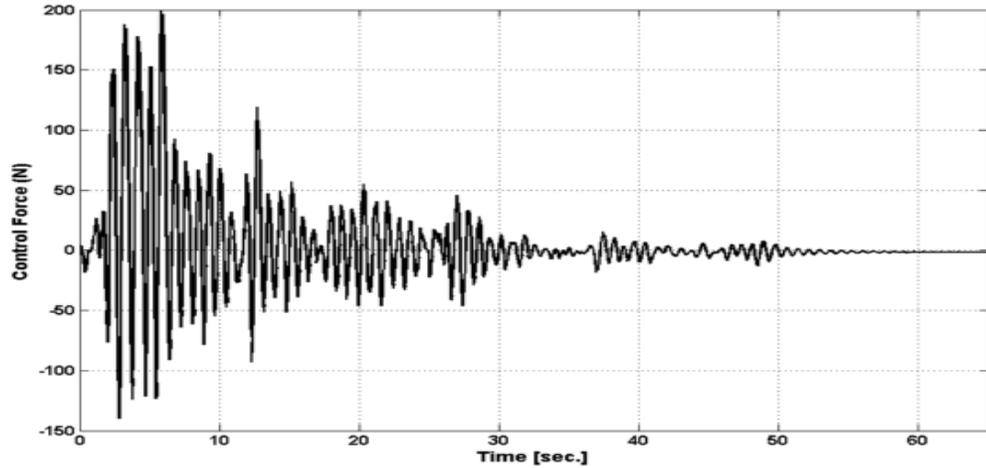
Figure 3-19 : 1<sup>st</sup> floor actuator force with 70% actuator fault
