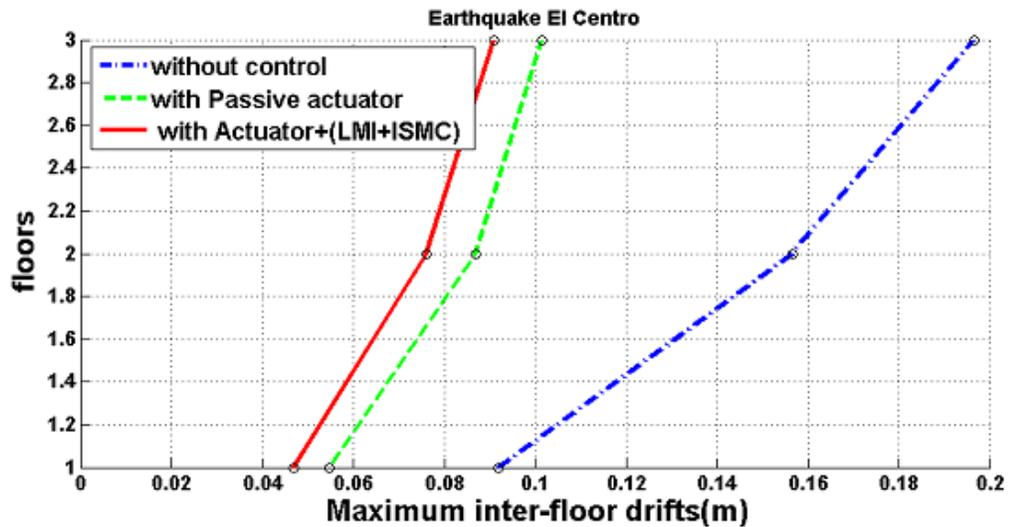
Figure 3-17 : Maximum inter-floor displacements without fault
