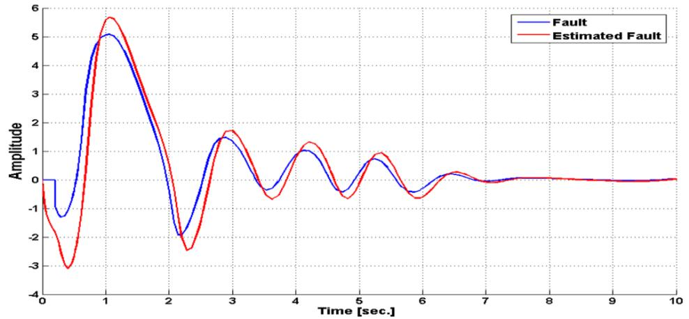
Figure 7-14: Estimated fault for 80% of 1<sup>st</sup> subsystem actuator fault ( $\eta_1=4.5$ )
