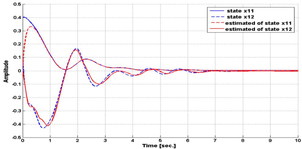
Figure 7-15: Estimated state for 80% of 1<sup>st</sup> subsystem actuator fault ( $\eta_1=4.5$ )
