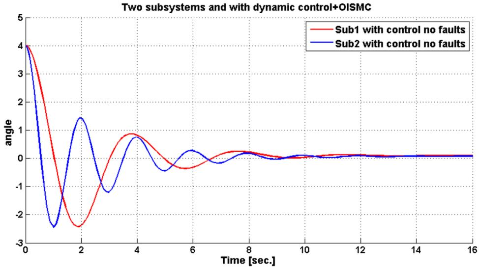
Figure 6-4: The inverted pendula angles with controller and no faults
