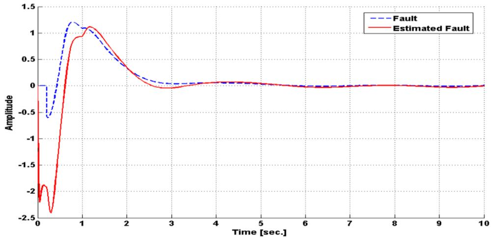
Figure 7-5 : Estimated fault with 50% of 1<sup>st</sup> subsystem actuator fault ( $\eta_1=10$ )
