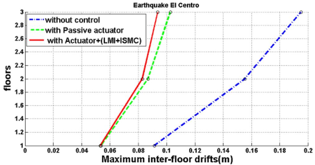
Figure 3-24 : Maximum inter-floor displacements without fault
