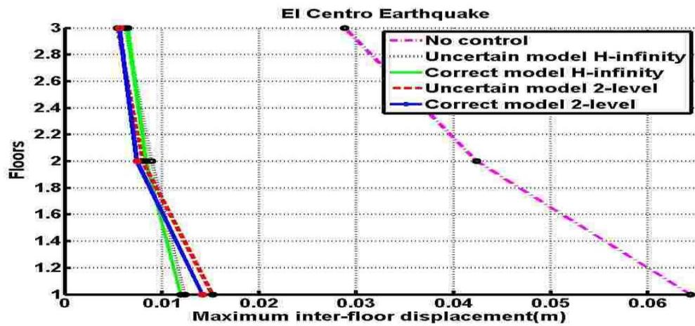
Figure 2-25: Maximum displacements: 10% mismatched & correct models with  $H_\infty$  & two-level control
