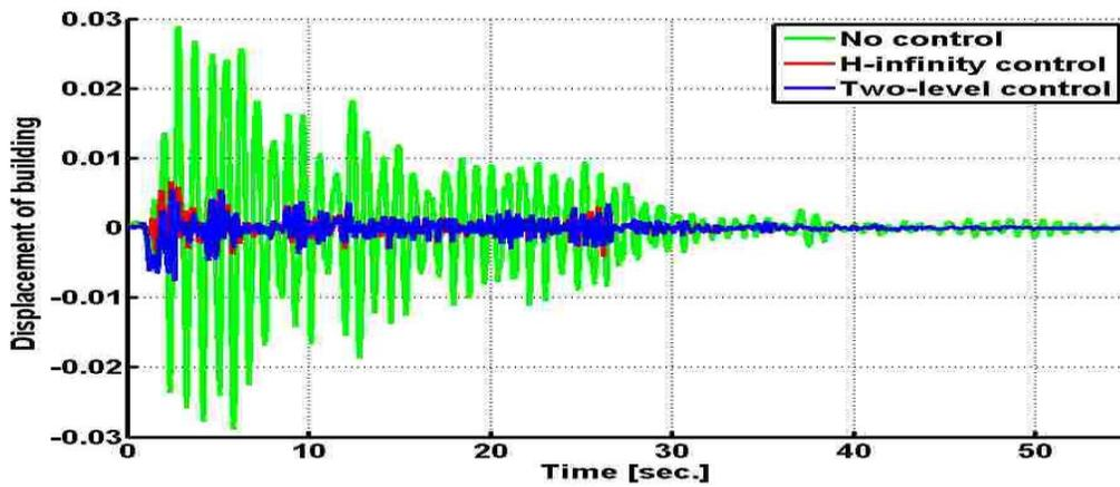
Figure 2-16: 3<sup>rd</sup> floor displacements
