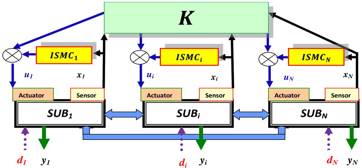
Figure 3-4: Control of inter-connected systems via LMI + ISMC (One shot)
