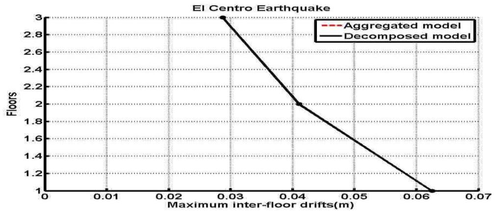
Figure 2-13: Displacements for both aggregated and distributed systems
