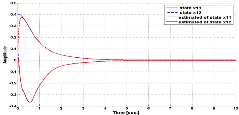
Figure 7-6: Estimated state for 50% of 1<sup>st</sup> subsystem actuator fault ( $\eta_1=10$ )
