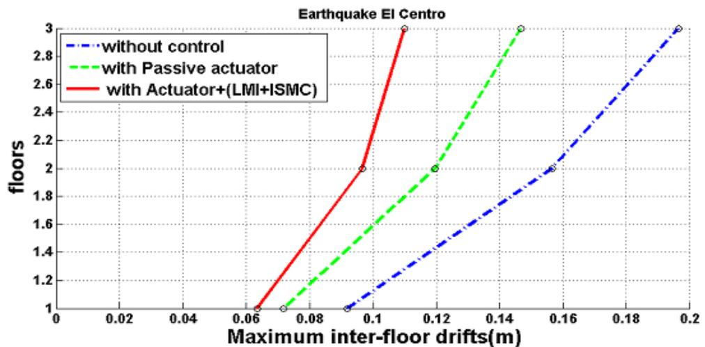
Figure 3-16: Maximum inter-floor displacement: 1<sup>st</sup>, 2<sup>nd</sup> and 3<sup>rd</sup> floor 70% actuator fault
