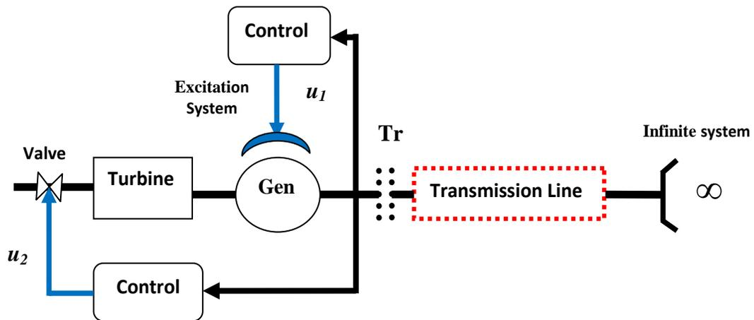
Figure 5-2: Single machine connected to infinite bus system
