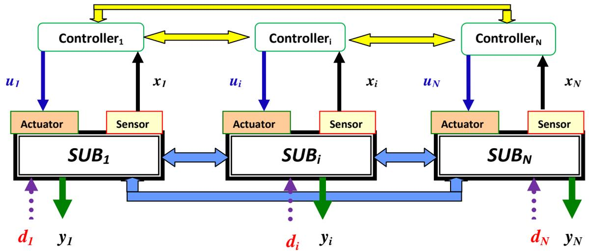
Figure 1-4: De-centralized overlapping control of inter-connected systems
