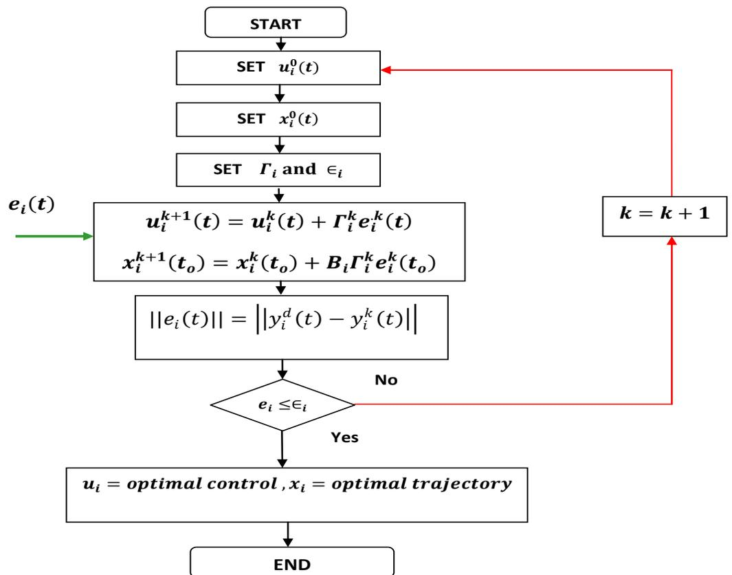
Figure 2-6: Flowchart of the algorithm of de-centralized iterative learning control for inter-connected systems with unknown interconnections
