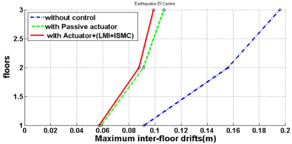
Figure 3-27 : Maximum inter-floor displacement: 1<sup>st</sup> floor 70% actuator fault
