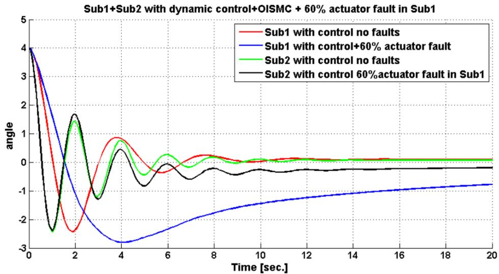
Figure 6-5: 1<sup>st</sup> subsystem with controller and 60% actuator fault
