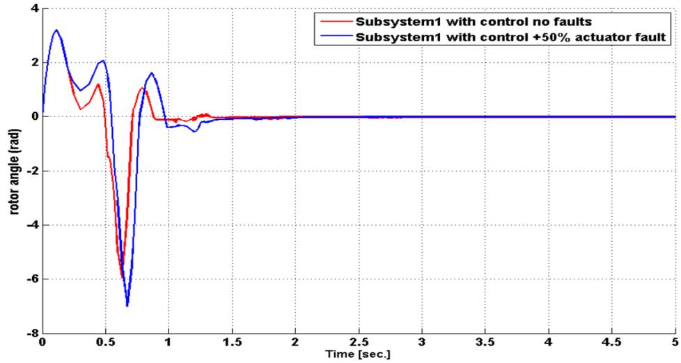
Figure 5-6 : 1<sup>st</sup> subsystem with AOISM and 50% actuator faults in only in 1<sup>st</sup> subsystem
