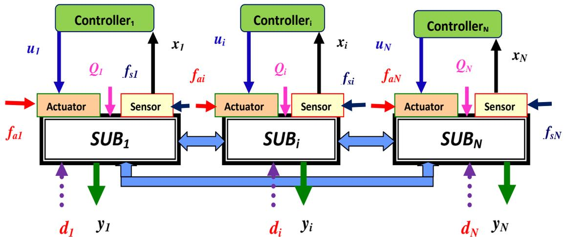
Figure 1-8: Types of faults in inter-connected systems
