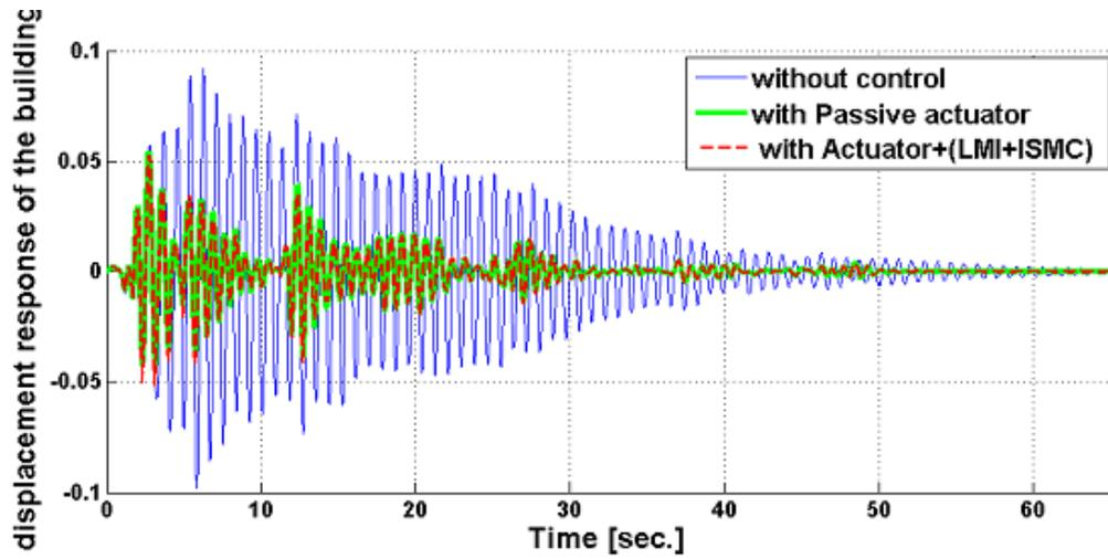
Figure 3-7: 1<sup>st</sup> floor displacements
