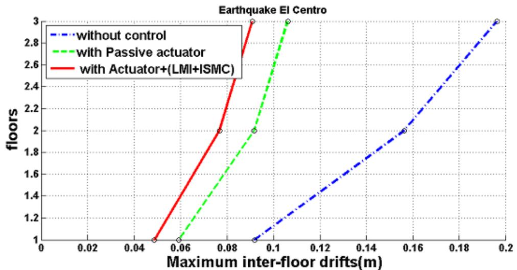
Figure 3-20 : Maximum inter-floor displacement: 1<sup>st</sup> floor 70% actuator fault
