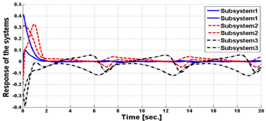
Figure 4-9: Three subsystems with controls and with 50% actuator fault in 1<sup>st</sup>, 2<sup>nd</sup> and 3<sup>rd</sup> subsystems
