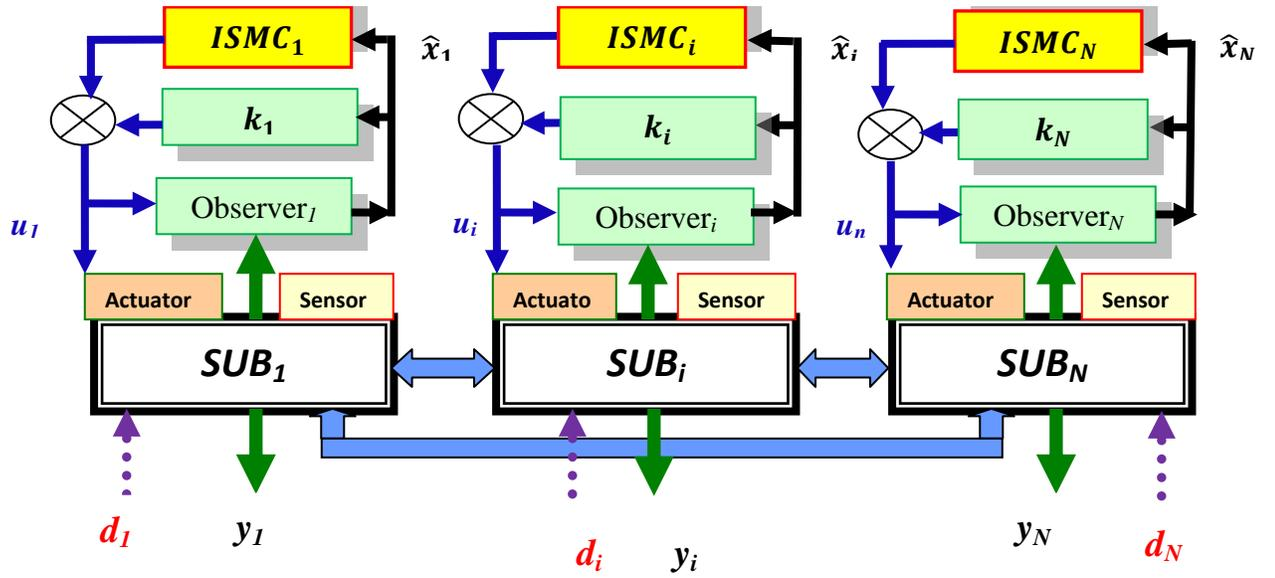
Figure 4-1: Output control of inter-connected systems via LMI+ISMC
