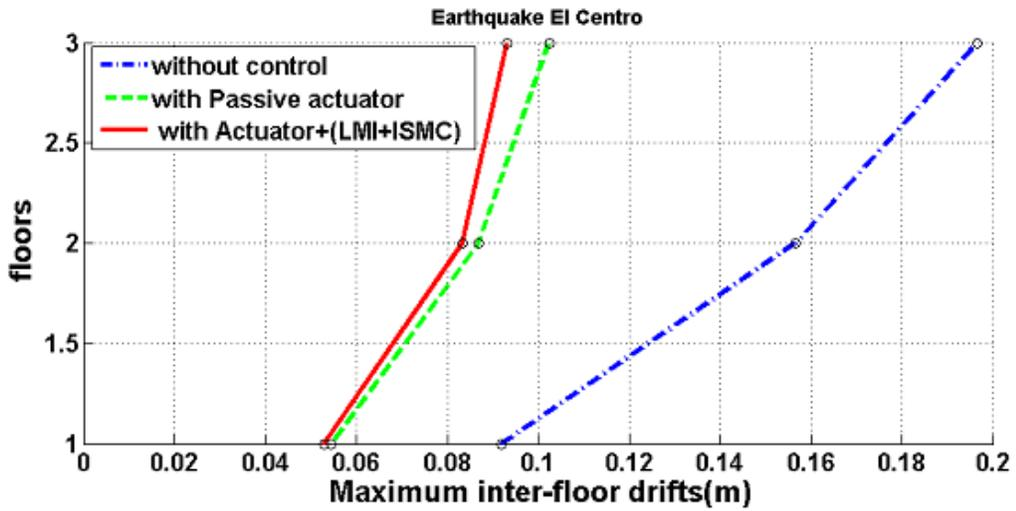
Figure 3-10: Maximum inter-floor displacements without fault
