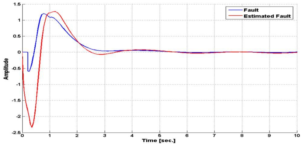
Figure 7-12: Estimated fault for 50% of 1<sup>st</sup> subsystem actuator fault ( $\eta_1=4.5$ )
