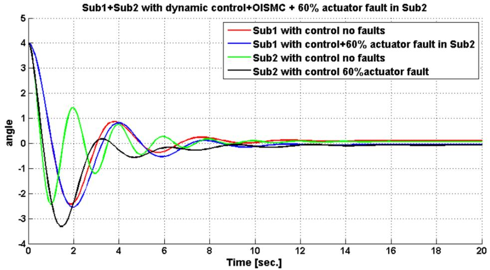
Figure 6-6: The 2<sup>nd</sup> subsystem with controller and 60% actuator fault
