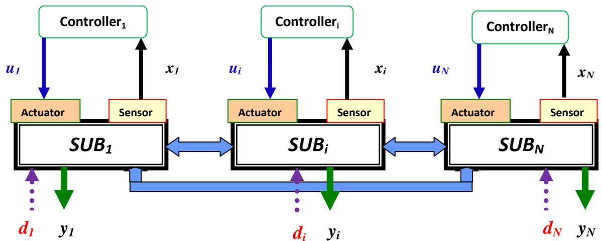
Figure 1-3: De-centralized control of inter-connected systems
