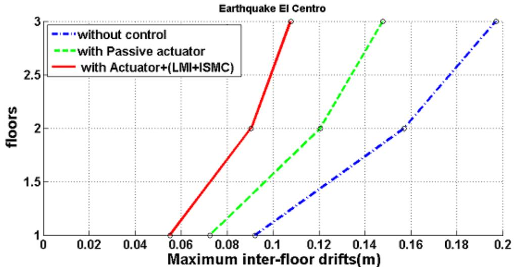
Figure 3-30 : Maximum inter-floor displacement: 1<sup>st</sup>, 2<sup>nd</sup> and 3<sup>rd</sup> floor 70% actuator fault
