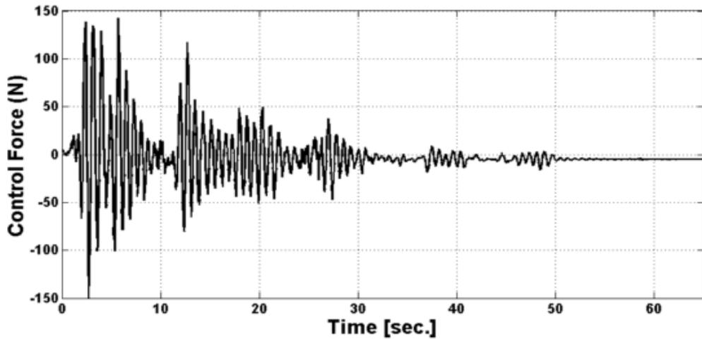
Figure 3-25 : 1<sup>st</sup> floor control force with no faults
