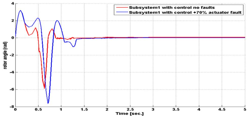
Figure 5-7 : 1<sup>st</sup> subsystem with AOISM and 70% actuator faults in only in 1<sup>st</sup> subsystem
