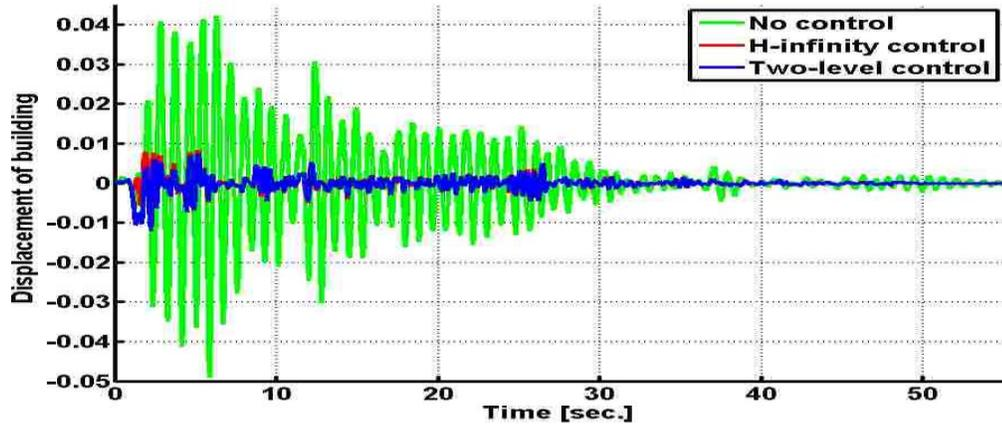
Figure 2-15: 2<sup>nd</sup> floor displacements
