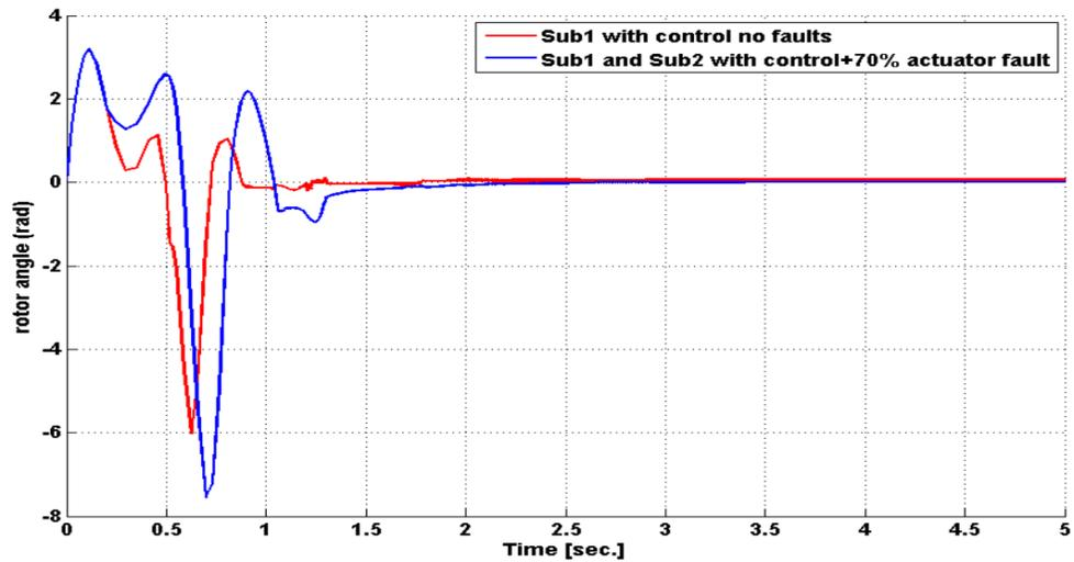
Figure 5-9 : Two subsystems with AOISM with 70% actuator faults in all subsystems
