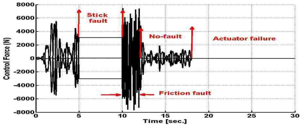
Figure 2-19: 1<sup>st</sup> floor actuator malfunction and failure
