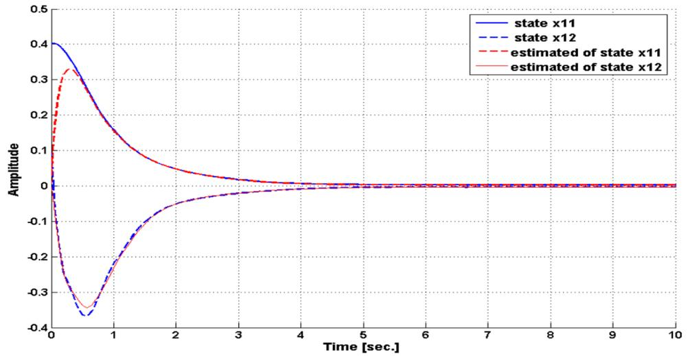
Figure 7-13: Estimated state for 50% of 1<sup>st</sup> subsystem actuator fault ( $\eta_1=4.5$ )
