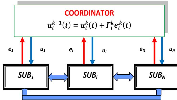
Figure 2-5: De-centralized iterative learning control for inter-connected systems with unknown interconnections
