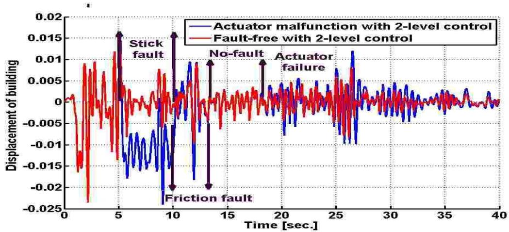
Figure 2-20: 1<sup>st</sup> floor displacement (two-level control and actuator faults)
