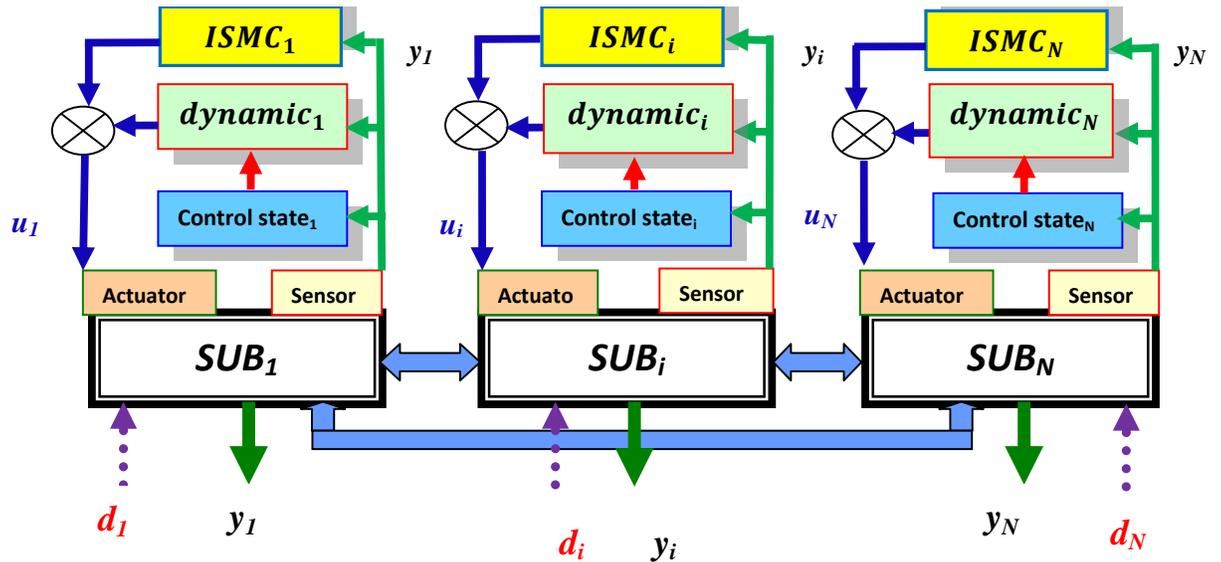
Figure 6-1: Dynamic output control of inter-connected systems via LMI+AOISM
