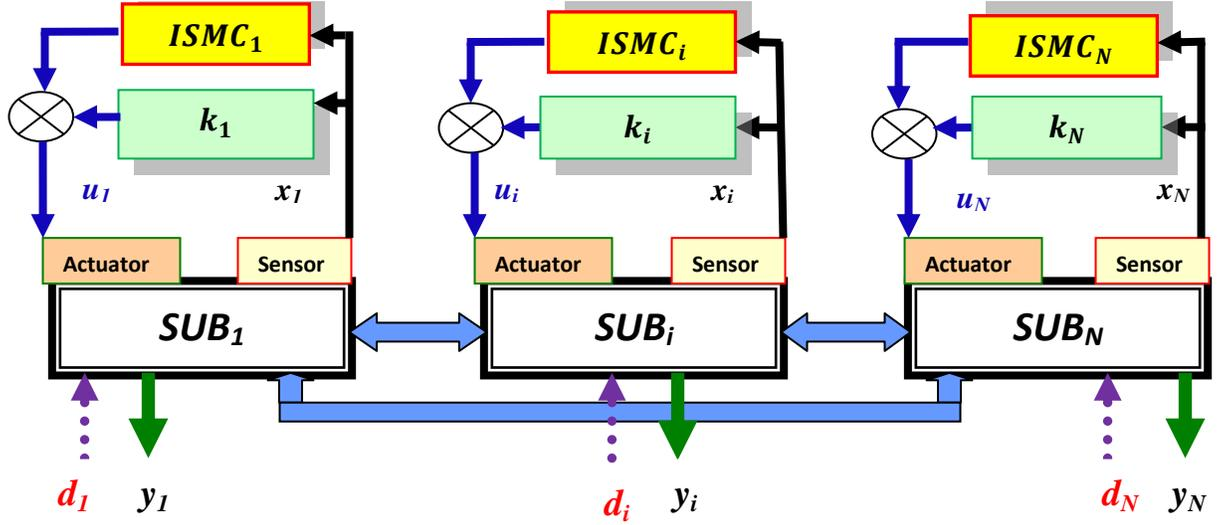
Figure 3-3: Control of inter-connected systems via LMI + ISMC subsystem by subsystem
