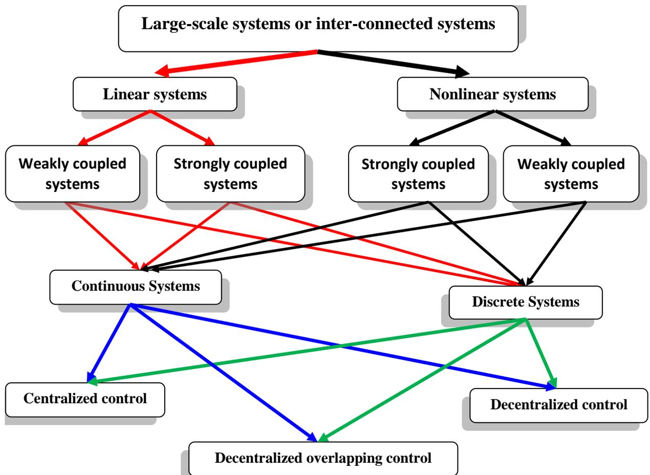
Figure 1-1: Classification of inter-connected systems and types of control
