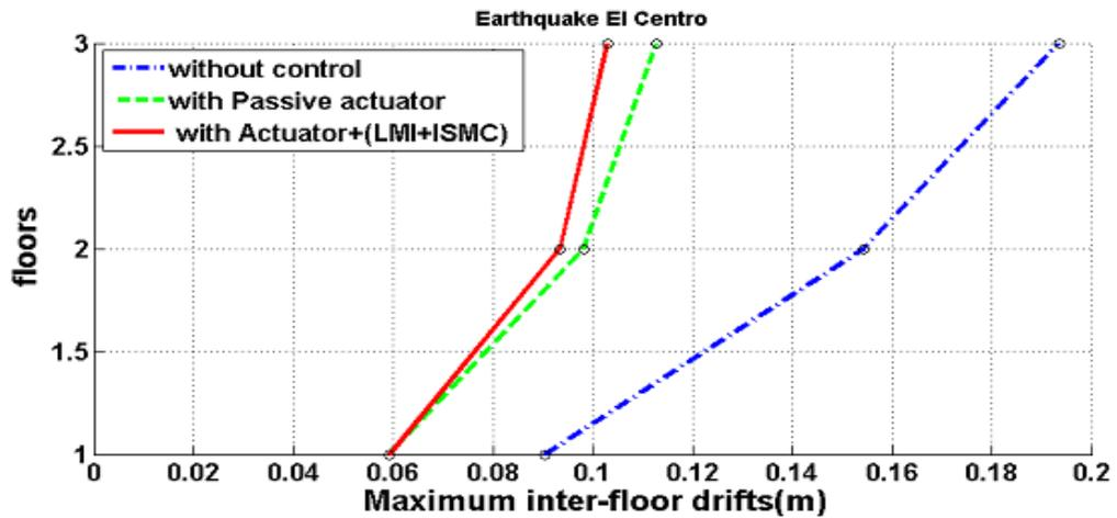
Figure 3-29 : Maximum inter-floor displacement: 1<sup>st</sup> and 2<sup>nd</sup> floor 70% actuator fault
