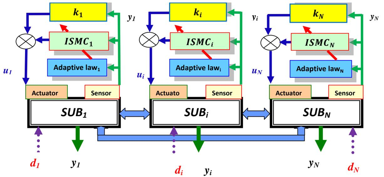
Figure 5-1: Static output control of inter-connected systems via LMI+AOISM
