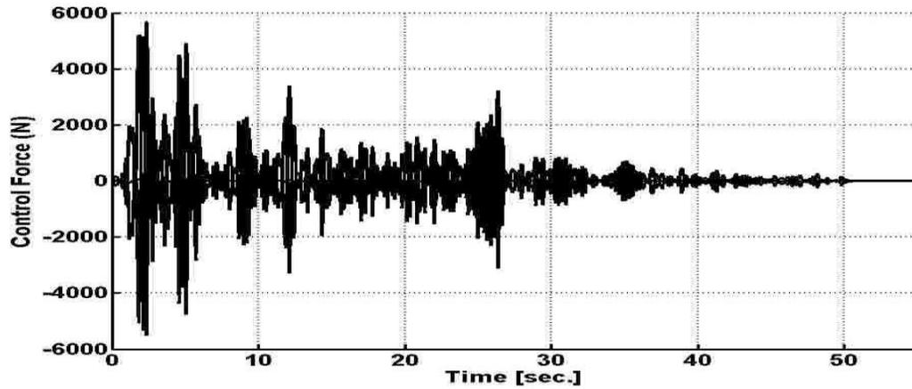
Figure 2-18: 1<sup>st</sup> floor actuator force with no faults
