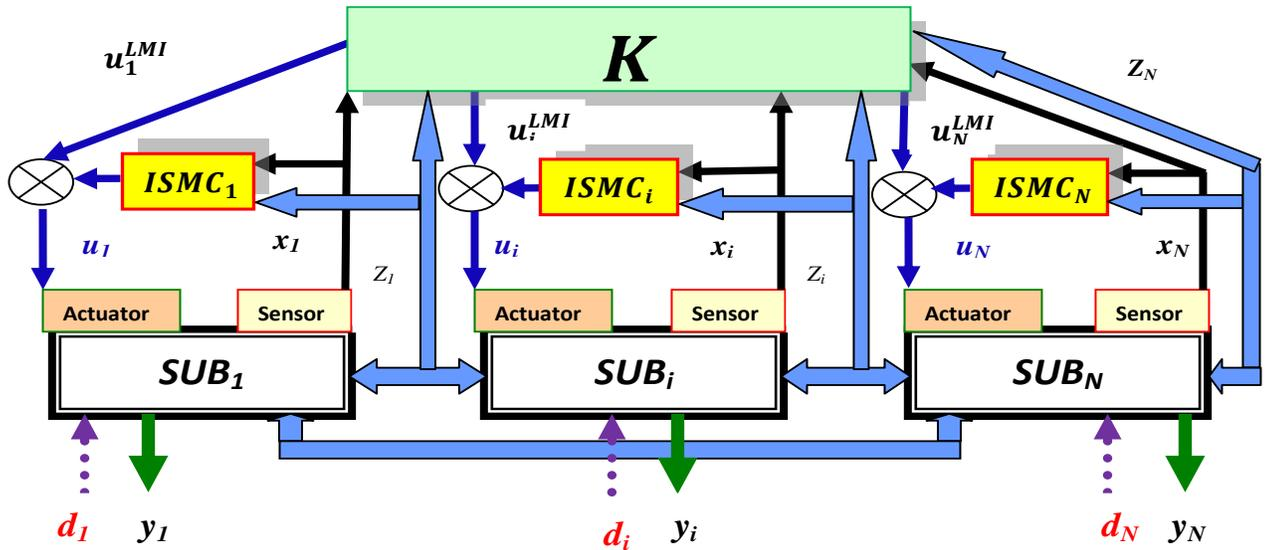
Figure 3-5: Control of inter-connected systems (known interactions) via LMI + ISMC one shot system
