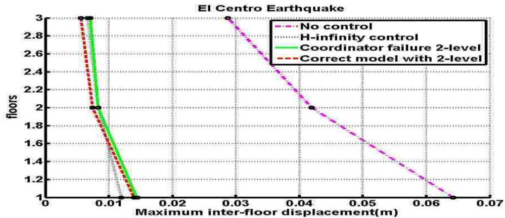
Figure 2-24: Maximum inter-floor displacement: Coordinator failure
