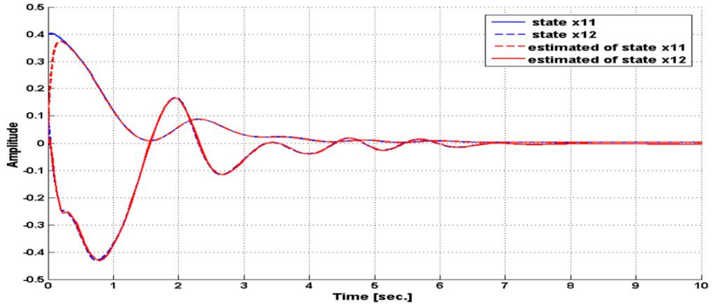
Figure 7-9 : Estimated state for 80% of 1<sup>st</sup> subsystem actuator fault (  $\eta_1=10$  )
