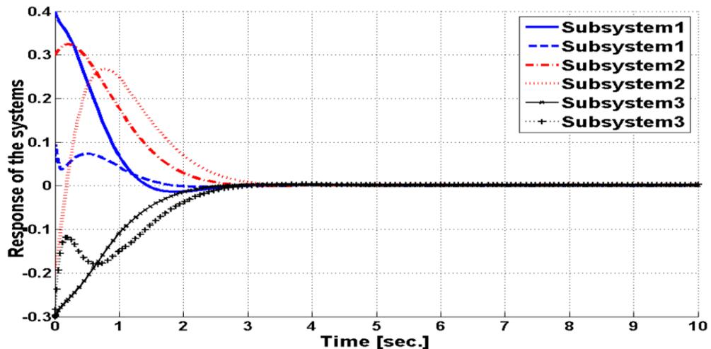
Figure 4-11: Three linear subsystems with controls but no faults and no interconnections or uncertainties
