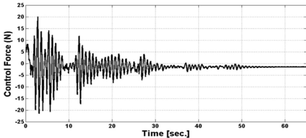
Figure 3-12: 1<sup>st</sup> floor actuator force with 70% actuator fault
