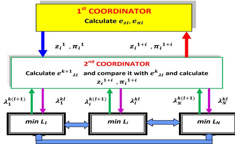
Figure 2-4: Three-level prediction principle controller
