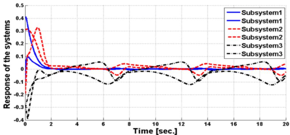
Figure 4-18 : Three subsystems with controls and with 50% actuator faults in the 1<sup>st</sup>, 2<sup>nd</sup> and 3<sup>rd</sup> subsystems
