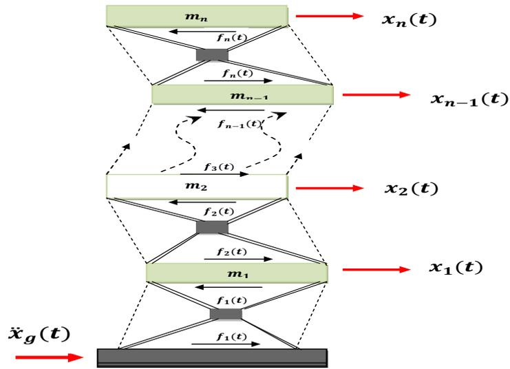
Figure 3-6: The effects of one dimensional earthquake on building of  $n$ -floor
