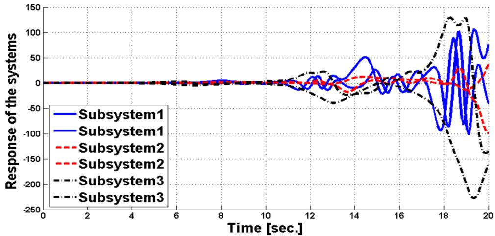
Figure 4-10 : Three subsystems with controls and with 70% actuator fault of 1<sup>st</sup>, 2<sup>nd</sup> and 3<sup>rd</sup> subsystems
