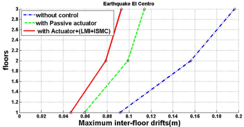
Figure 3-22 : Maximum inter-floor displacement: 1<sup>st</sup> and 2<sup>nd</sup> floor 70% actuator fault
