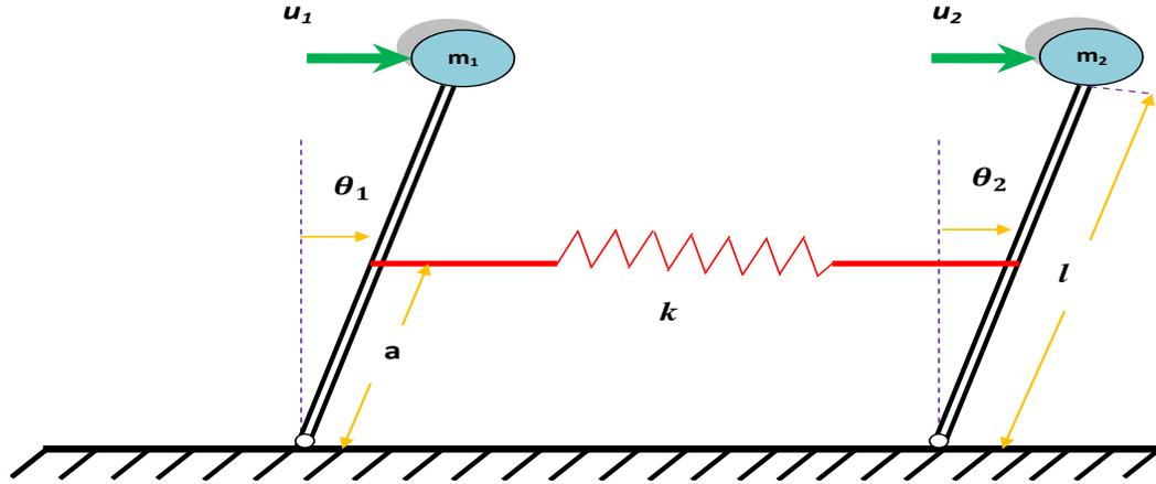
Figure 6-2 : Two coupled inverted pendula
