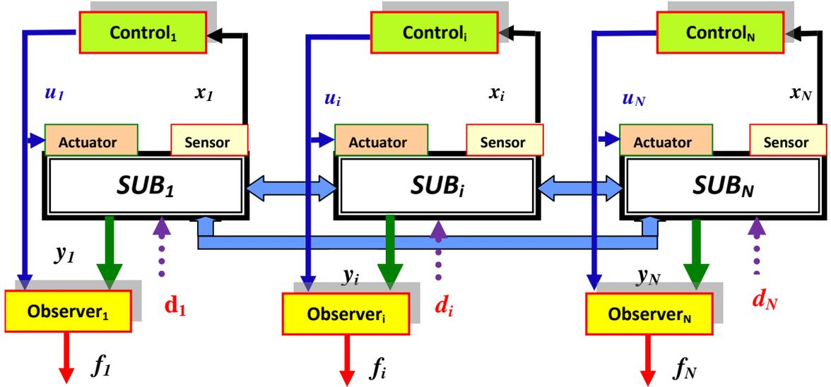
Figure 7-1: Fault estimation in inter-connected system via subsystem observers
