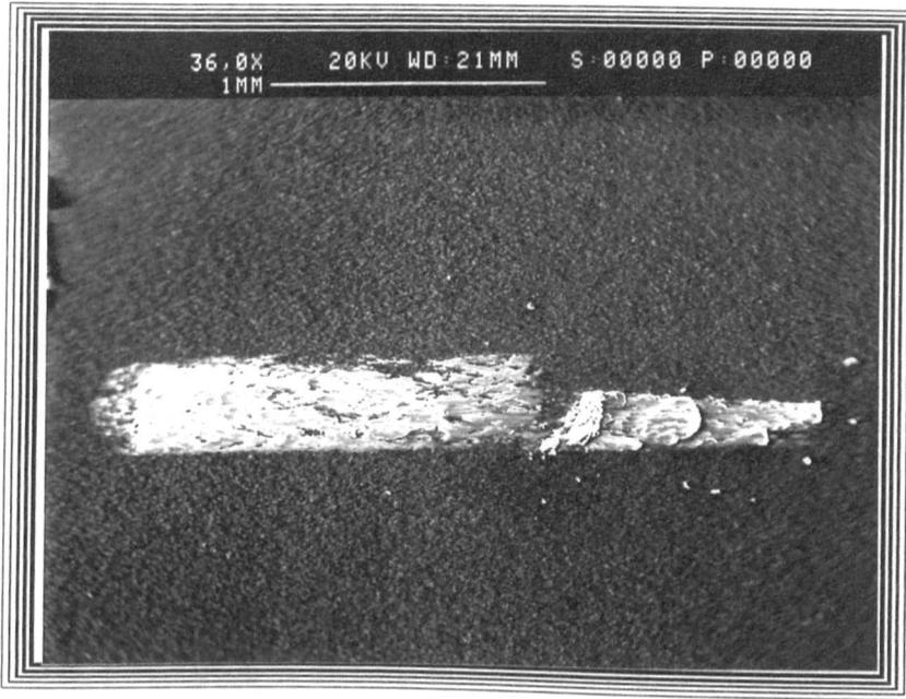
Figure 5.4 (a) Adherent aluminium on polycrystalline diamond (Syndax)
