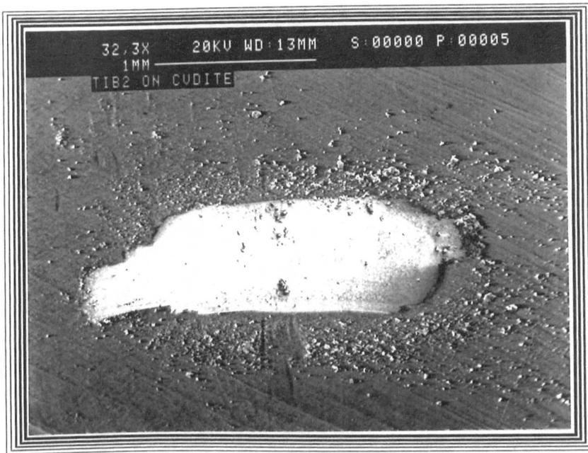
Figure 5.6 (a) Wear track produced by TiB<sub>2</sub> slider on CVDite after 3500 traversals
