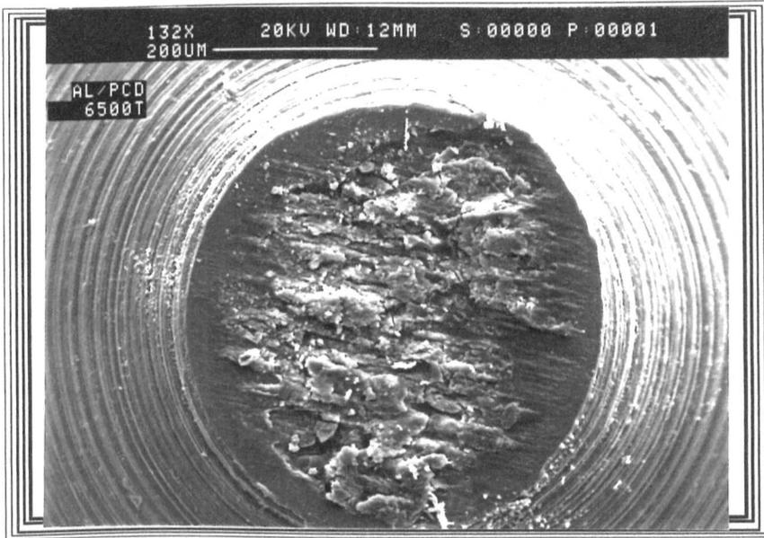
Figure 5.12 Debris layer formed on the blunted tip of an aluminium slider after 6500 traversals on Syndite
