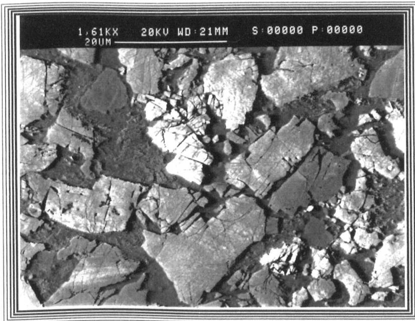
Figure 5.8 (b) High magnification of the above track showing the formation of cracks in the diamond particles
