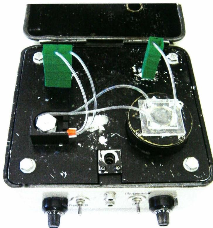
*Figure 2.3 Photograph showing the portable chemiluminescence detection system designed in-house. The microfluidic connections can be seen with peristaltic pump tubing connected directly from the sample/reagent containers to the microfluidic device located above the PMT. Further peristaltic pump tubing connects the microfluidic channels to the waste container. The reagent, sample and waste containers are covered with black tape when the box is operational to reduce interference.*
