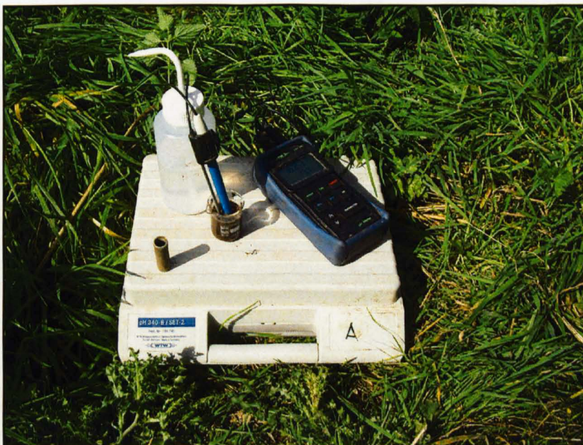
Figure 3.10: Equipment used for the measurement of temperature and pH in the field.
