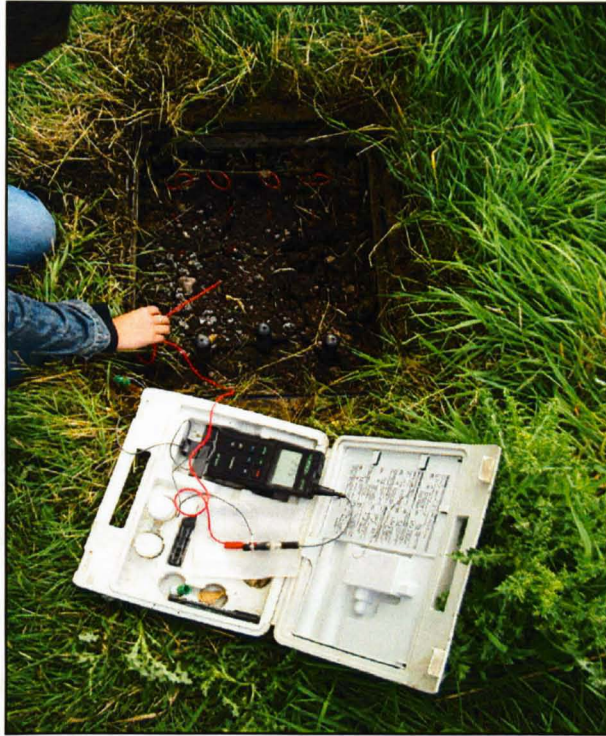
Figure 3.8: Acquisition of redox potential readings in the field at Hatfield Moor.
