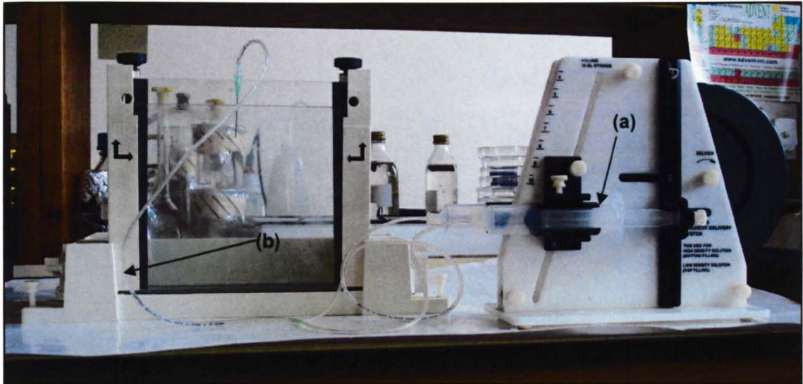
Figure 5.7: Cam operated gradient delivery system mixes high and low density solutions to create the denaturing gradient. Syringes (a) used to deliver the gel to the casting tray through the Y-shaped tubes (b).
