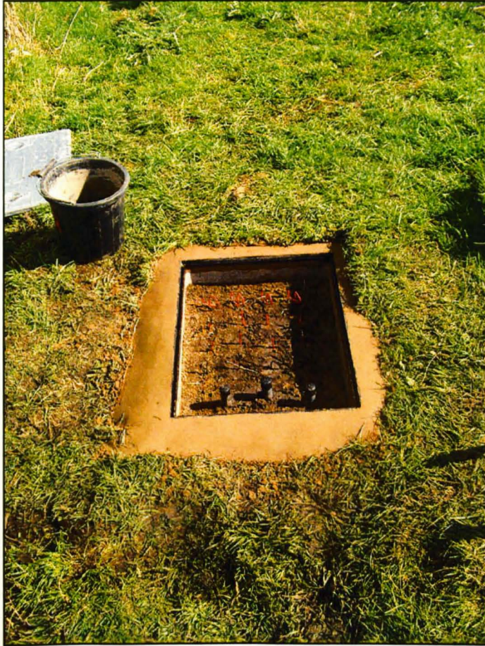
Figure 3.1: Photograph showing the monitoring point (100 cm x 50 cm) at Hatfield Moor, including three piezometers and redox probes at different depths.
