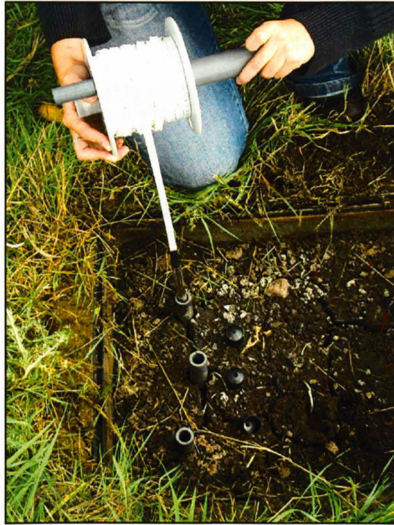
Figure 3.4: Acquisition of water level measurements using an acoustic dipper at Hatfield Moor
