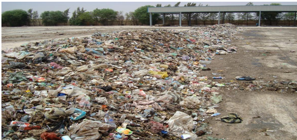
Figure 5-10: Compost pile in Sidi Al-Siah plant contaminated with inorganic waste
