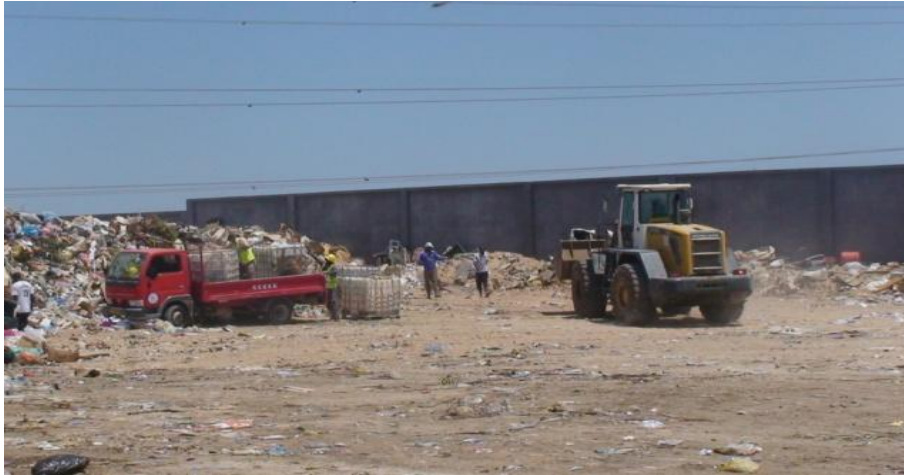
Figure 5-6: Practice at Tajora transfer station; loading from the ground
