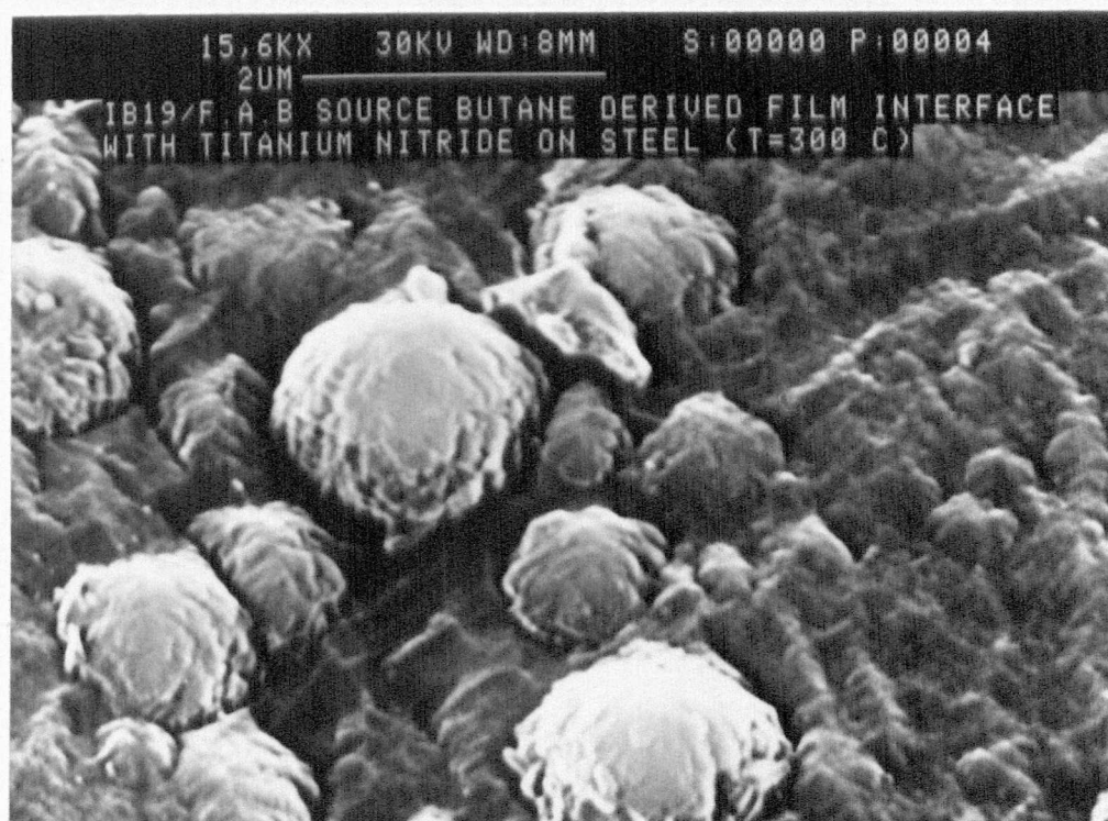
Fig. VI.32 : Scanning electron micrographs of particles observed on the interface TiN after debonding of DLC due to the annealing effect .
