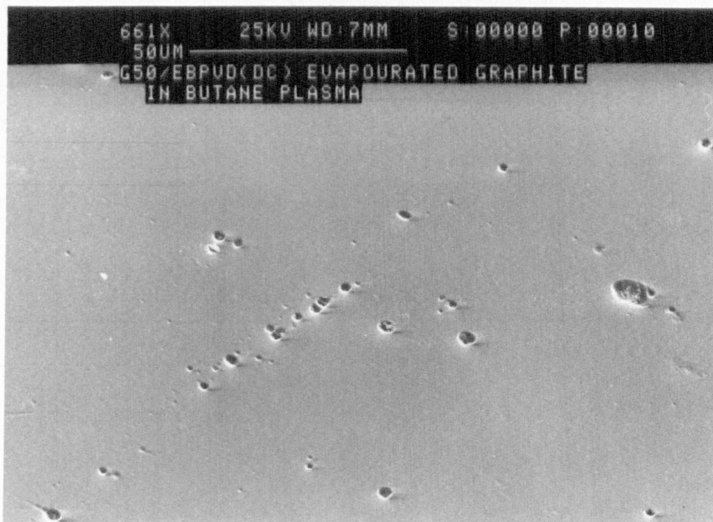
Fig.VII.5 Scanning electron plan micrograph of a carbon film produced on tool steel using d.c. EBPVD ( butane + graphite evaporation ).
