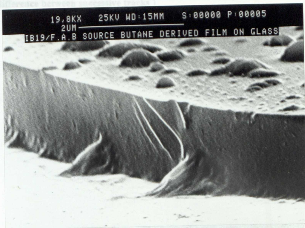
Fig. VI. 5 Scanning electron micrographs of FAB source carbon films; Top: Butane film on aluminium foil, bottom : on glass.
