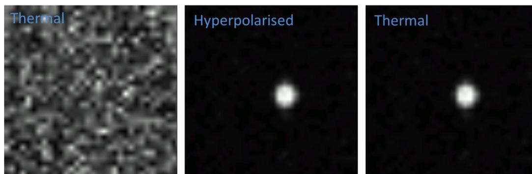
Figure 4.28:  $^{13}\text{C}$  MRI images acquired using a RARE pulse sequence. The three images from left to right are, thermally polarised single scan, hyperpolarised single scan and thermally polarised after 1100 scans.
