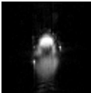
Figure 4.1:  $^1\text{H}$  MRI image acquired using an EPI sequence of a water sample. Very little optimisation has been completed and hence the image is poor.
