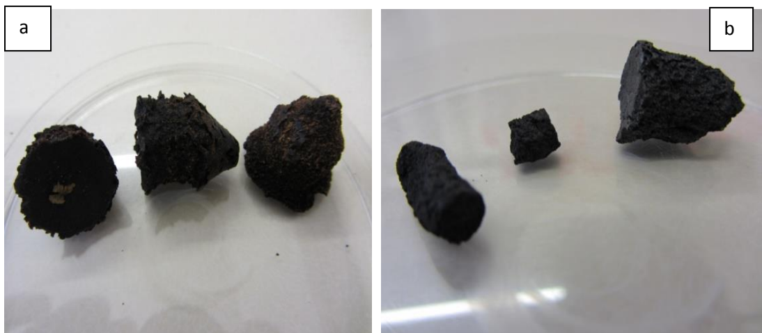
Figure 6.6: Photographs of (a) as-synthesized monolith (b) carbon monolith from evaporation-induced self-assembly using waste plant material as carbon precursor. The carbon monolith remained crack-free despite structural shrinkage during the high temperature carbonization.
