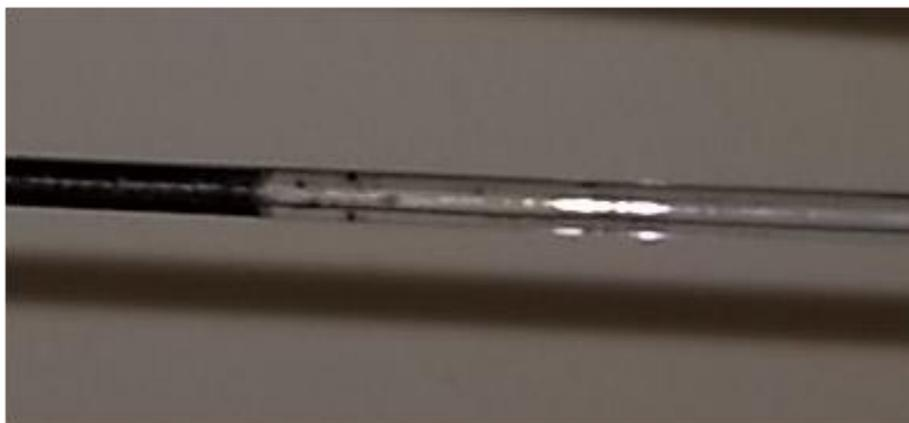
**Figure 3.7** A 25  $\mu\text{L}$  glass capillary containing a monolith coated in palladium from methods *monolith 2.3* and *palladium loading 2.12*.
