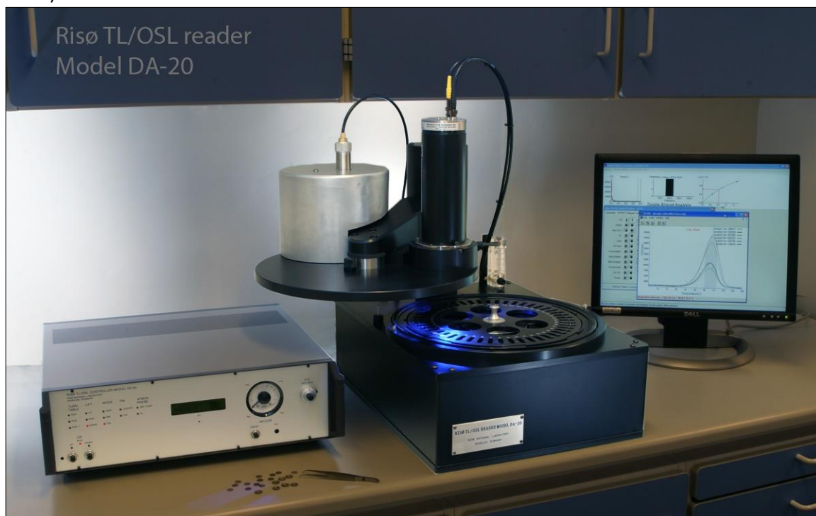
Figure APP 7.2 The Risø DA-20 luminescence reader (From Risø National Laboratory, 2009)
