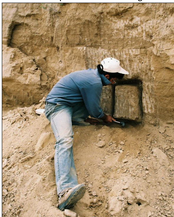
Figure 3.2 Carving out two adjacent block sediment samples from a Khuzestan river terrace exposure for OSL dating
