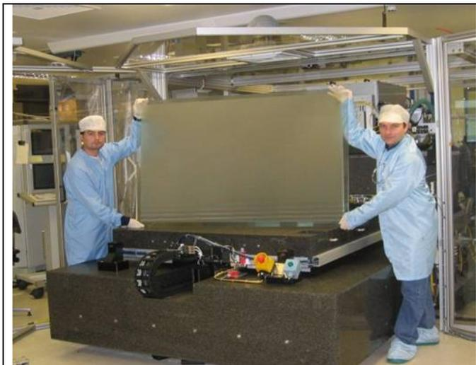
**Figure 114.** Demonstrator of large area micro-lens array. The author (right) and a colleague are presenting a 1 m x 1.5 m sample with a micro-lens array of  $\sim 500 \times 10^6$  lenses. The sample was produced on the Exitech PPM 601E system on which the sample rests.
