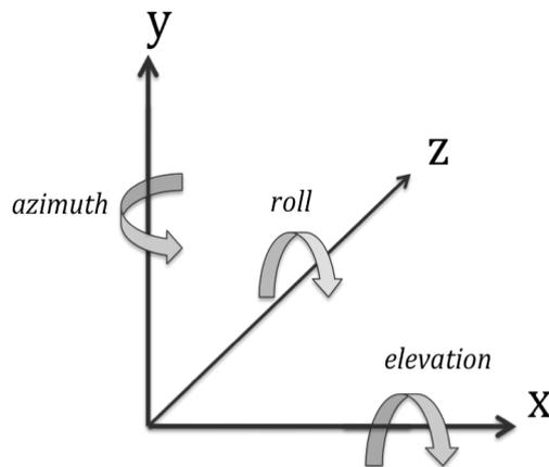
**Legend:** Each sensor's movements are measured in 3D space using three positional coordinates (x, y, z) and three orientation coordinates (azimuth, roll, elevation).
