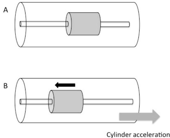
**Legend:** (A) the mass remains still when the cylinder is static or moving with constant velocity, (B) inertia causes the mass to lag behind when the cylinder accelerates. The relative distance moved by the mass, or the force of the supporting springs is proportional to the output signal.
