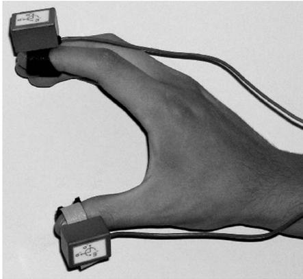
**Legend:** Lightweight KinetiSense motion sensors containing three accelerometers and three gyroscopes were placed on the subject's index finger and thumb but kinematic data was only extracted from the gyroscopes. *Image reproduced from Espay et al. 2011 with permission (Espay, Giuffrida et al., 2011).*
