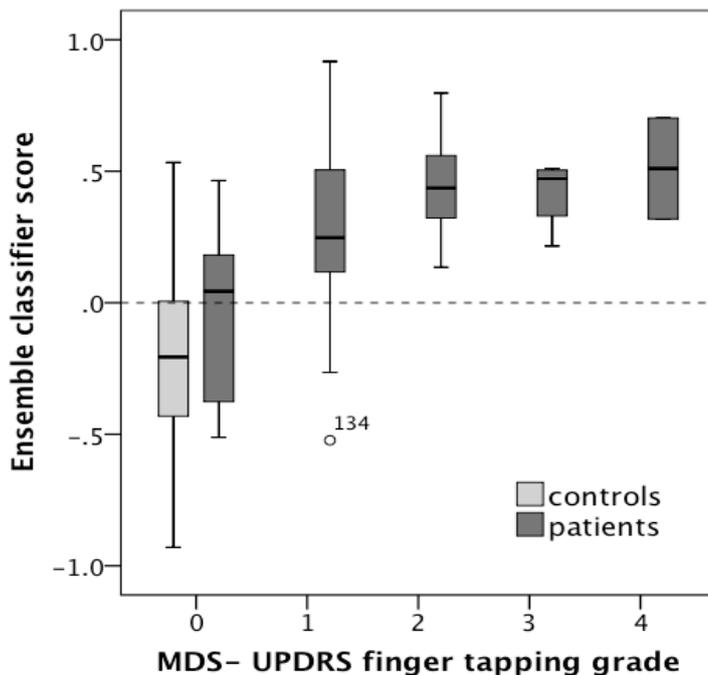
**Legend:** All PD and dominant HC data sets are presented. The horizontal dashed line at zero marks the decision threshold of the classifier solution. If the classifier score is  $>$  zero the data will be classified as PD and if the score is  $<$  zero it will be classified as HC. This figure shows that the majority of misclassified patients had a UPDRS FT grades of zero. It also shows that classifier solutions for grade zero PwPD are significantly higher than for grade zero controls.
