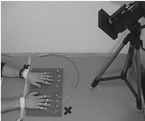
**Legend:** OKS equipment with reflective markers attached to the fingers and a table with metal stripes and bands around the wrists assure the reproducible hand-camera arrangement. *Image reproduced from Jobbagy et al. 2005 with permission. (Jobbagy, Harcos et al., 2005)*
