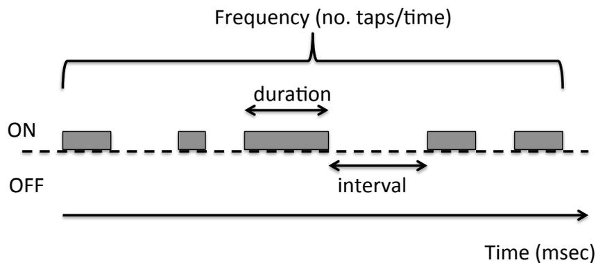
**Legend:** Schematic illustration of how contact sensors enable quantification of FT movement components such as frequency (number of taps per second), duration (period of time that sensor is on), interval (period of time between taps) and rhythm (variation in duration or interval).
