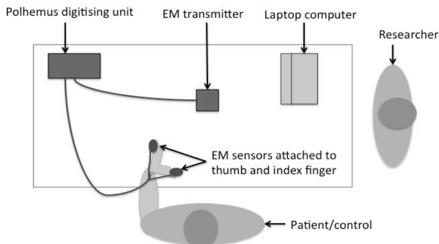
**Figure 19 Polhemus electromagnetic tracking system**
