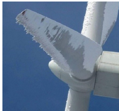
Figure 2-3 Icing on wind turbine blades (Anonymous, 2011b)
