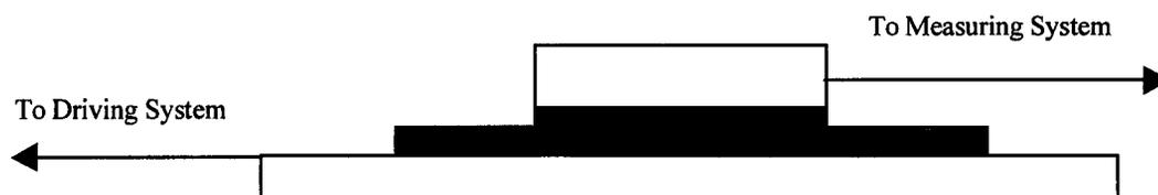
Figure 2.8. Dreby's principle for friction measurements
