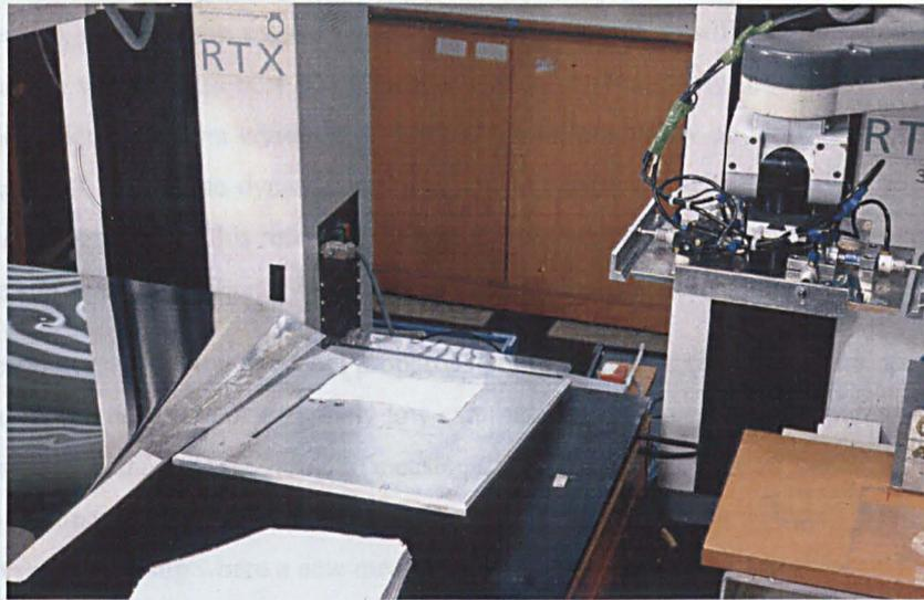
*Figure 1.2. Vibrating alignment table with pinching gripper at the Hull brief's assembly line*
