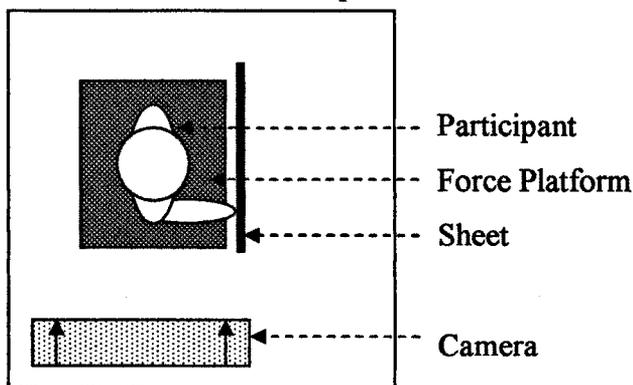
**Figure 2.2: Experimental area setup (top down-view)**
